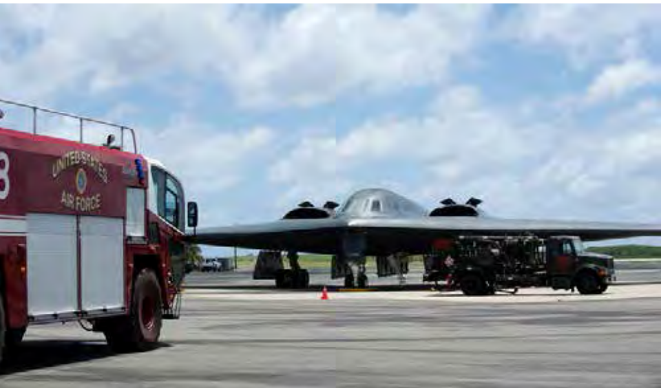
A U.S. Air Force B-2 Spirit, deployed from Whiteman Air Force Base, Mo., connects to a fuels truck during a hot-pit refueling at Wake Island Airfield Sept. 14, 2018. Hot-pit refueling is a technique where an aircraft lands and is refueled without shutting down its engines. These missions showcase the U.S. forces' ability to address a global security environment and demonstrates U.S. commitment to a free and open Indo-Pacific. (U.S. Air Force photo by Staff Sgt. Danielle Quilla)
