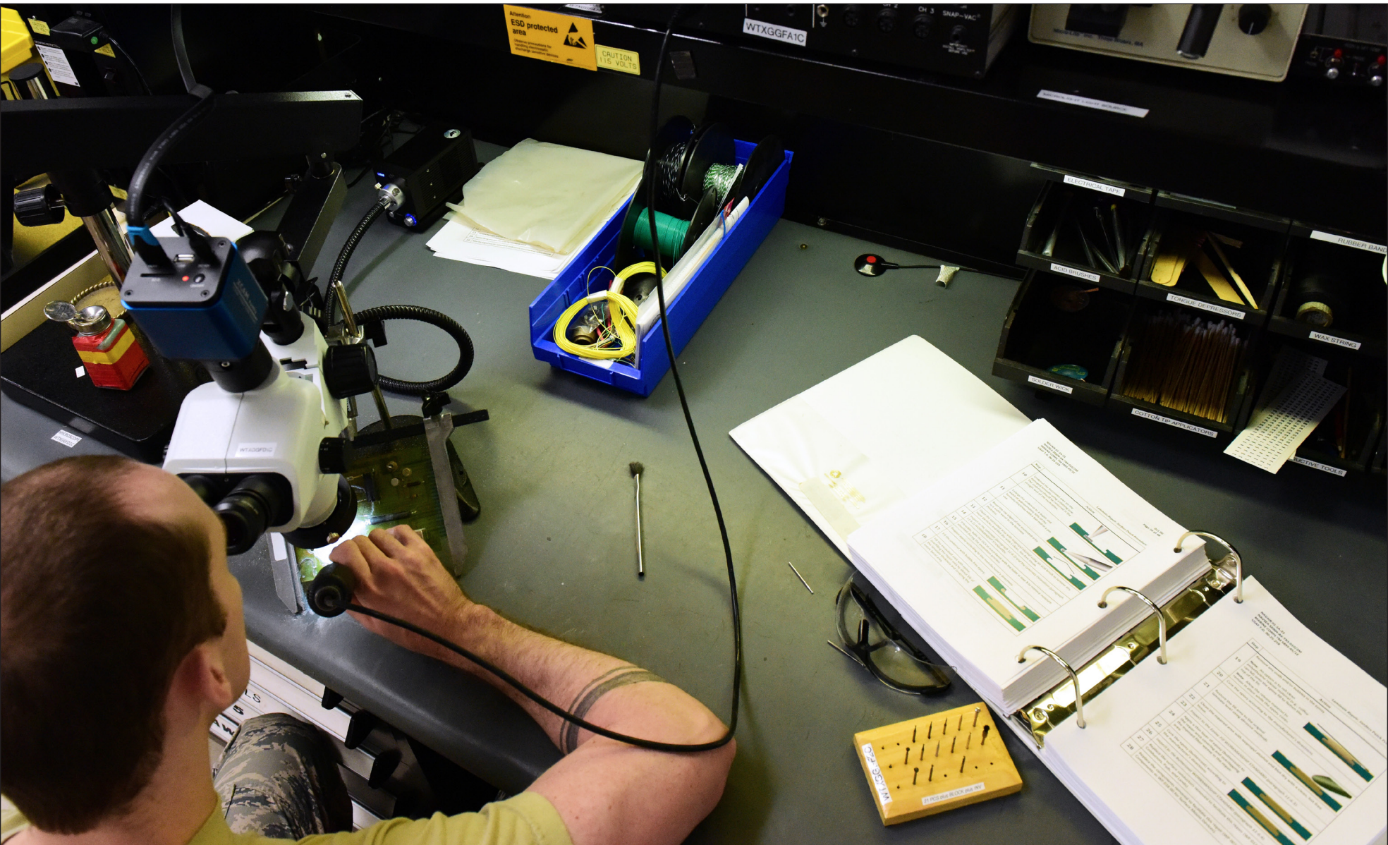
U.S. Air Force Staff Sgt. Christopher Lear, an Air Force Repair Enhancement Program technician assigned to the 509th Maintenance Group, removes the damaged layers from a circuit board at Whiteman Air Force Base, Missouri, on May 29, 2018. AFREP technicians attend certification courses at David-Monthan AFB, Arizona, to be qualified to perform electronic repairs.
