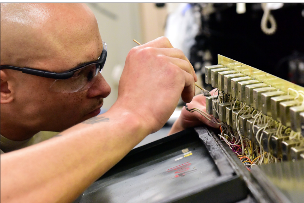
U.S. Air Force Tech. Sgt. Benjamin Sherrill, an Air Force Repair Enhancement Program technician assigned to the 509th Maintenance Group, cleans a damaged circuit board from a power control unit on May 29, 2018. It is worth $70,000 and is part of the munition lift trailer at Whiteman Air Force Base, Missouri.
