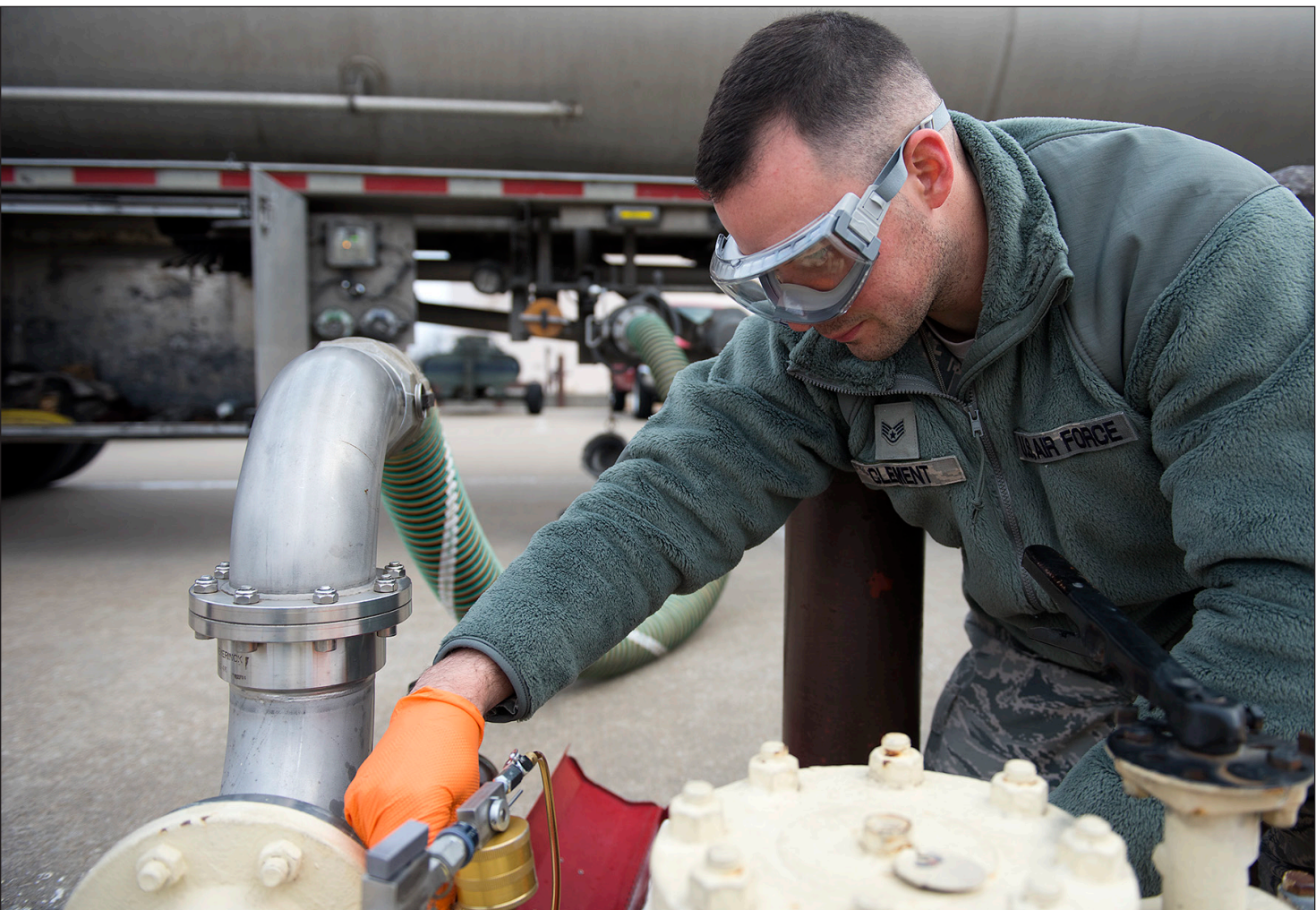
U.S. Air Force Staff Sgt. Kyle Clement, a fuels lab technician assigned to the 509th Logistics Readiness Squadron, takes samples of fuel at Whiteman Air Force Base, Mo., March 8, 2018. The fuels technicians pull samples and test the fuel around base for water, additives and sediment like rocks, dirt or other particles.
