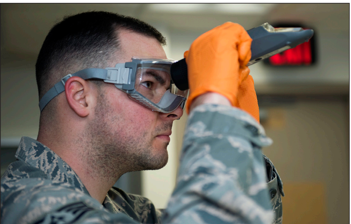
U.S. Air Force Staff Sgt. Kyle Clement, a fuels lab technician assigned to the 509th Logistics Readiness Squadron, tests the fuel at Whiteman Air Force Base, Mo., March 8, 2018. The fuels technicians pull samples and test the fuel around Whiteman to ensure it is safe to use in an aircraft or any fuel-based system.
