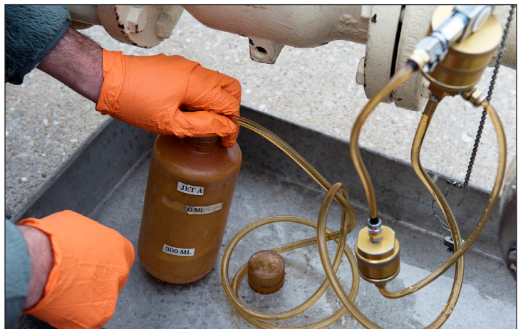
U.S. Air Force Staff Sgt. Kyle Clement, a fuels lab technician assigned to the 509th Logistics Readiness Squadron, takes samples of Jet A fuel at Whiteman Air Force Base, Mo., March 8, 2018. There are additives in the Jet A fuel and the fuels technicians perform specific tests to ensure the amount of additives are within their passing limits as well as making sure there isn’t an abundance of water and particulates in the fuel.
