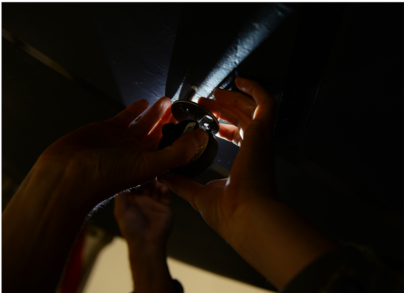
Staff Sgt. James B. Finn, a signature diagnostics technician assigned to the 509th Bomb Wing, uses a step height gauge during an inspection of a B-2 Stealth Bomber on Oct. 16, 2018 at Whiteman Air Force Base, Missouri. Members of the signature diagnostics section perform various inspections of the aircraft after maintenance is performed to ensure the fidelity of the aircraft's protective capabilities. (U.S. Air Force photo by Staff Sgt. Kayla White)
