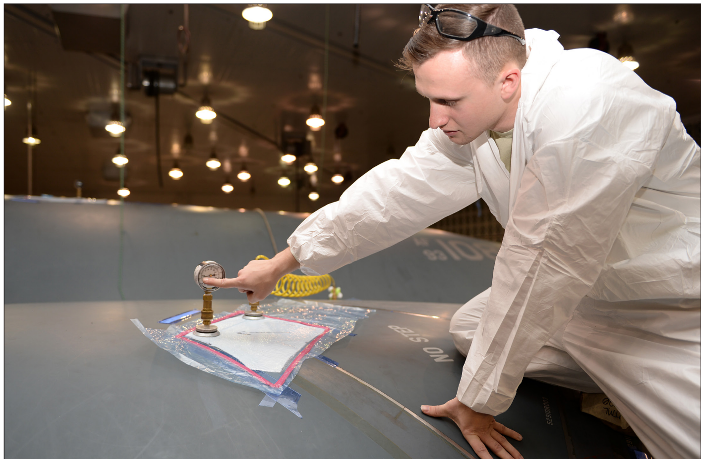
Senior Airman Austin K. Choate, a low-observable maintenance technician assigned to the 509th Maintenance Group, displays the tools used to vacuum seal tape on the B-2 Stealth Bomber on Oct. 24, 2018 at Whiteman Air Force Base, Missouri. Choate performs regular maintenance to ensure the fidelity of the aircraft. (U.S. Air Force photo by Staff Sgt. Kayla White)
