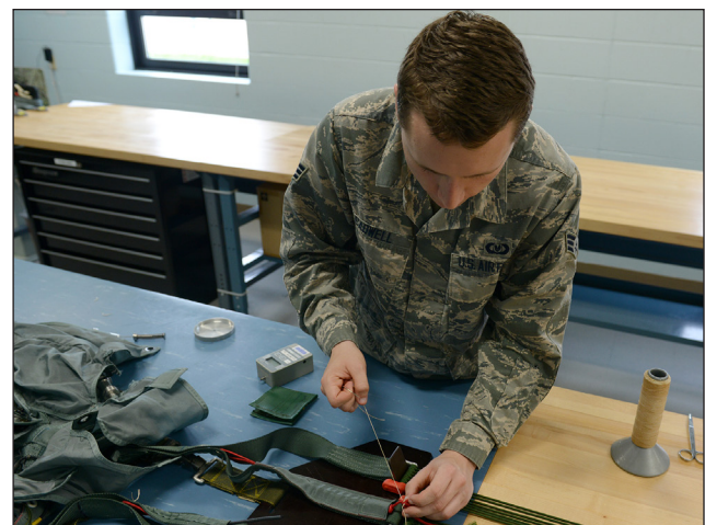
U.S. Air Force Senior Airman Thomas Cadwell, an aircrew flight equipment technician assigned to the 509th Operations Support Squadron, inspects a four-line release at Whiteman Air Force Base, Mo., Aug. 21, 2017. The four-line release is used after the pilot has ejected and needs to steer the parachute to keep it from landing in an unsafe area.
