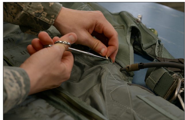
U.S. Air Force Senior Airman Thomas Cadwell, an aircrew flight equipment technician assigned to the 509th Operations Support Squadron, inspects the oxygen bottle attached to a parachute at Whiteman Air Force Base, Mo., Aug. 21, 2017. If a pilot ejects at a high altitude with less oxygen, he will need to pull the oxygen bottle cord which will release oxygen through a tube connected to his helmet.
