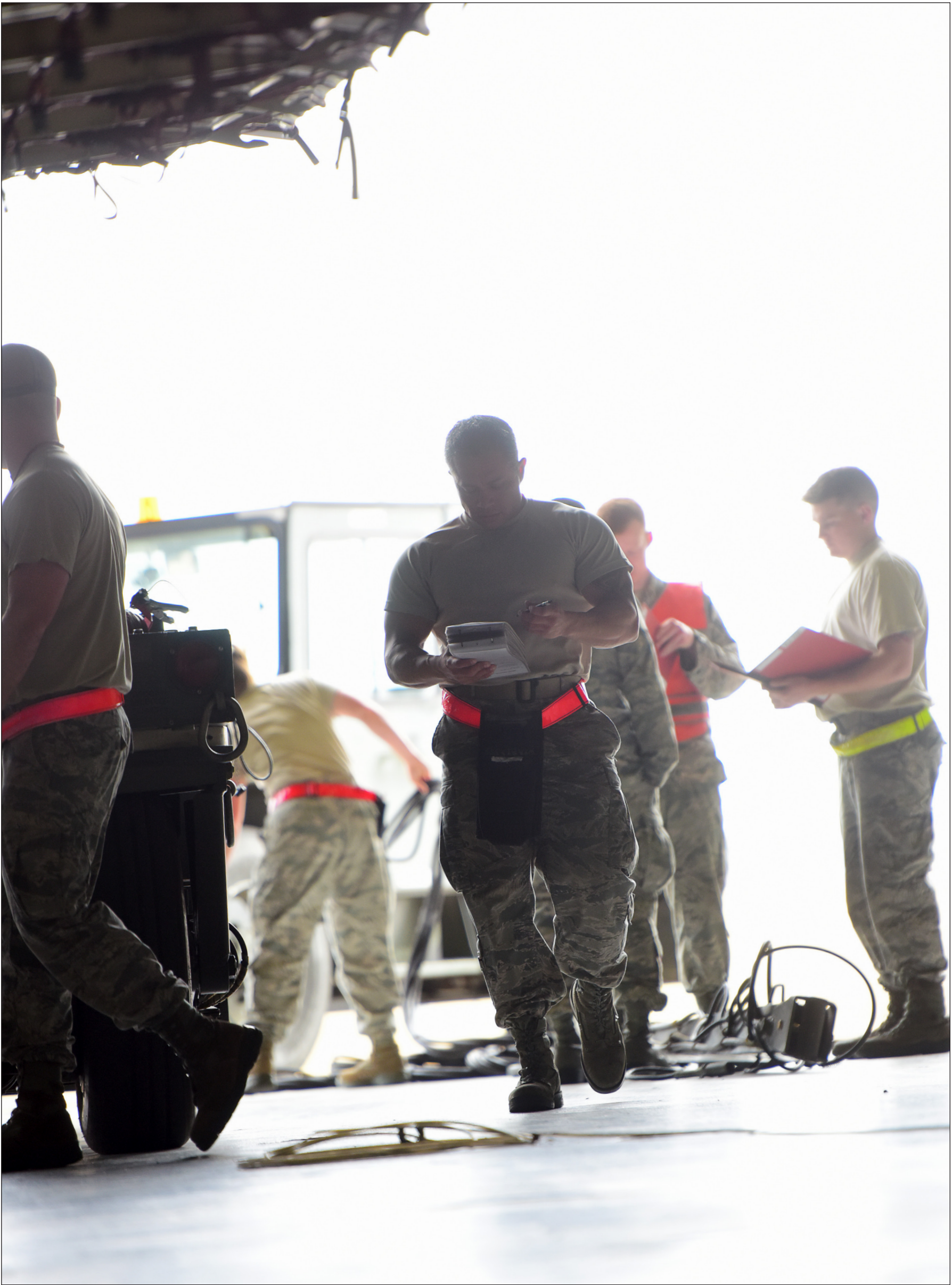
U.S. Air Force photo/Airman 1st Class Jazmin Smith Crew chiefs and weapons specialists assigned to the 509th and 131st Aircraft Maintenance Squadrons look over the munitions handling unit (MHU)-204 trailer for defects while performing a visual inspection of the assets during a no-notice operational readiness exercise at Whiteman Air Force Base, Mo., Feb. 28, 2017. During the exercise, Total-Force Integrated Airmen were tasked with executing Whiteman's strategic deterrence mission while validating operational readiness.
