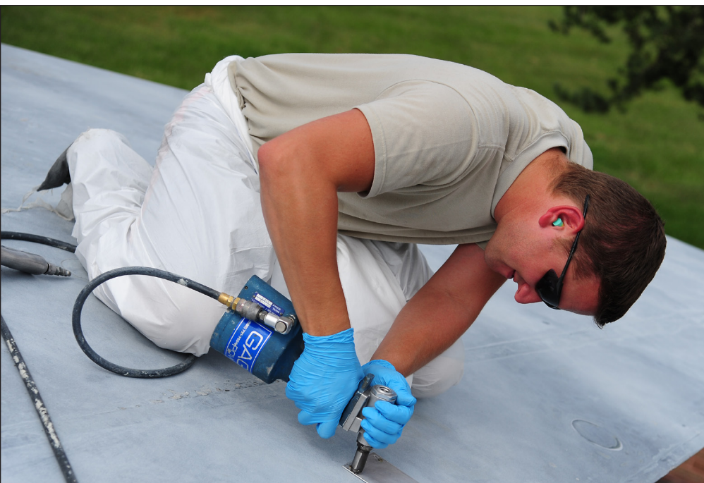
U.S. Air Force Tech Sgt. Nicholas Fonzo, a low observable technician from the 509th Maintenance Squadron, repairs corrosion damage on an FB-111A General Dynamics Aardvark static display at Whiteman Air Force Base, Mo., Sept. 13, 2016. The static displays on base require maintenance due to weather and wildlife as needed.
