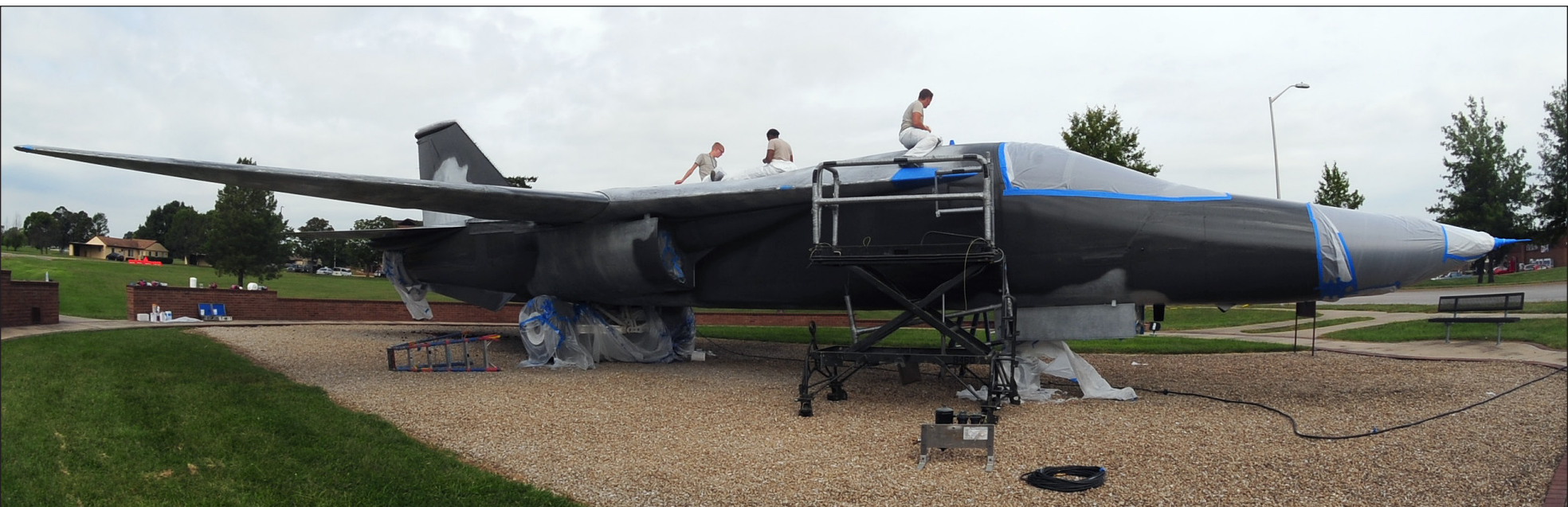
Low observable technicians from the 509th Maintenance Squadron tape off sections of an FB-111A General Dynamics Aardvark static display prior to repainting it at Whiteman Air Force Base, Mo., Sept. 13, 2016. During the restoration process, the aircraft was sanded, primed, repainted and received corrosion maintenance.
