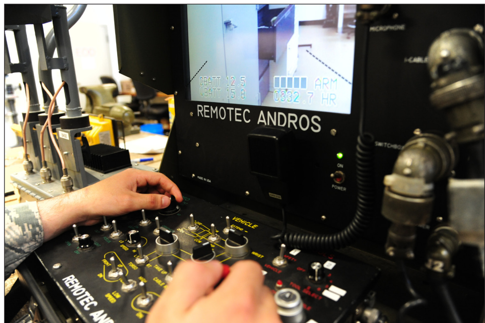
U.S. Air Force Airman 1st Class Conner Walsh, a 509th Civil Engineer Squadron explosive ordnance disposal (EOD) team member, uses an F6A robot controller at Whiteman Air Force Base, Mo., May 10, 2016. The robots are the primary means of handling explosive ordnances to eliminate potential harm to EOD members.
