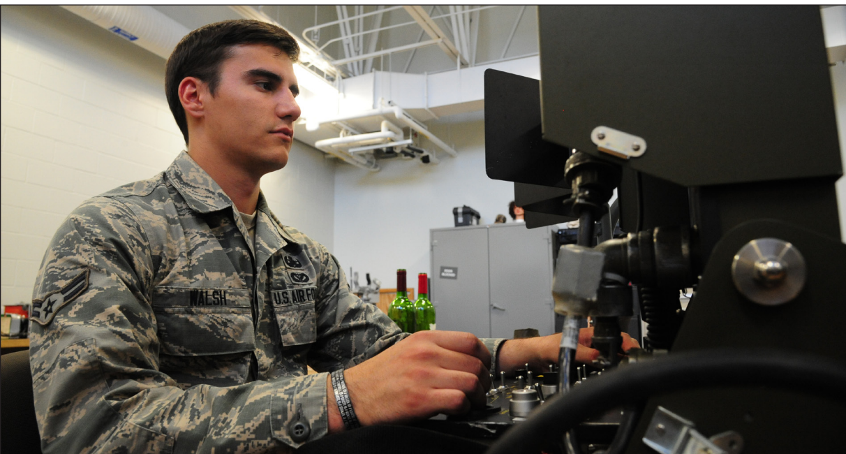
U.S. Air Force Airman 1st Class Connor Walsh, a 509th Civil Engineer Squadron explosive ordnance disposal team member, operates an F6A robot controller at Whiteman Air Force Base, Mo., May 10, 2016. The controller enables the robot to maneuver around different obstacles as well as disarm explosive devices.
