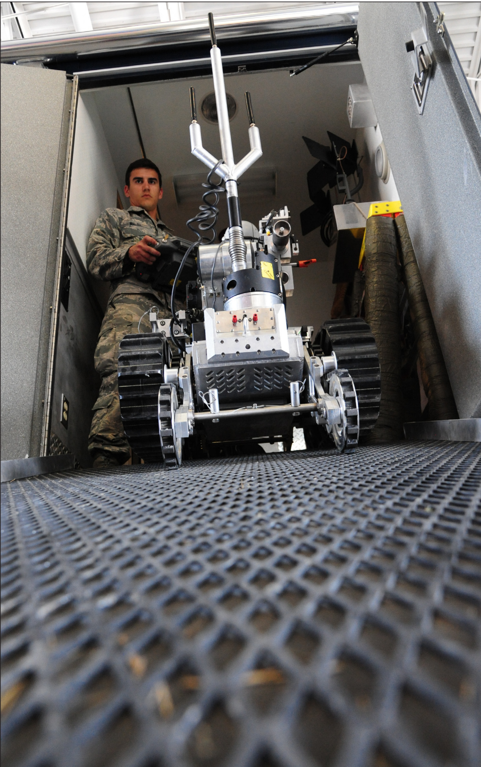
U.S. Air Force Airman 1st Class Connor Walsh, a 509th Civil Engineer Squadron explosive ordnance disposal (EOD) team member, controls an HD2 robot on an EOD response vehicle at Whiteman Air Force Base, Mo., May 10, 2016. When the EOD team receives a response call regarding a suspicious package, they deploy a robot downrange to investigate the device.
