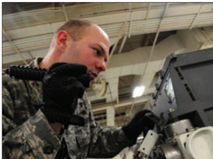
U.S. Air Force Senior Airman Nicholas McClary, a weapons specialist from the 509th Munitions Squadron, inspects and verifies data plates on a rotary launcher assembly at Whiteman Air Force Base, Mo., Feb. 12, 2016. The rotary launcher is inspected to ensure the components are compatible with the weapons system prior to being loaded.
