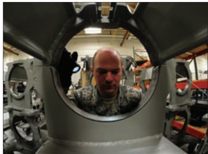
U.S. Air Force Senior Airman Nicholas McClary, a weapons specialist from the 509th Munitions Squadron, performs a serviceability check on an H1125A bomb handling truck at Whiteman Air Force Base, Mo., Feb. 12, 2016. Each component of the handling gear is inspected thoroughly to ensure it's operational before using it to install a weapon.
