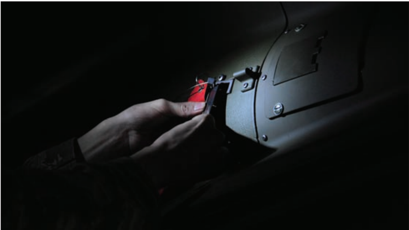
ABOVE: U.S. Air Force Staff Sgt. Paul Wiese, a 393rd Aircraft Maintenance Unit load crew member secures the wing release lanyard on a GBU-28 B/B during a quarterly weapons load competition at Whiteman Air Force Base, Mo., Jan. 13, 2016. The competitions are held quarterly to test the crew's ability to load weapons in a timely and precise manner.
