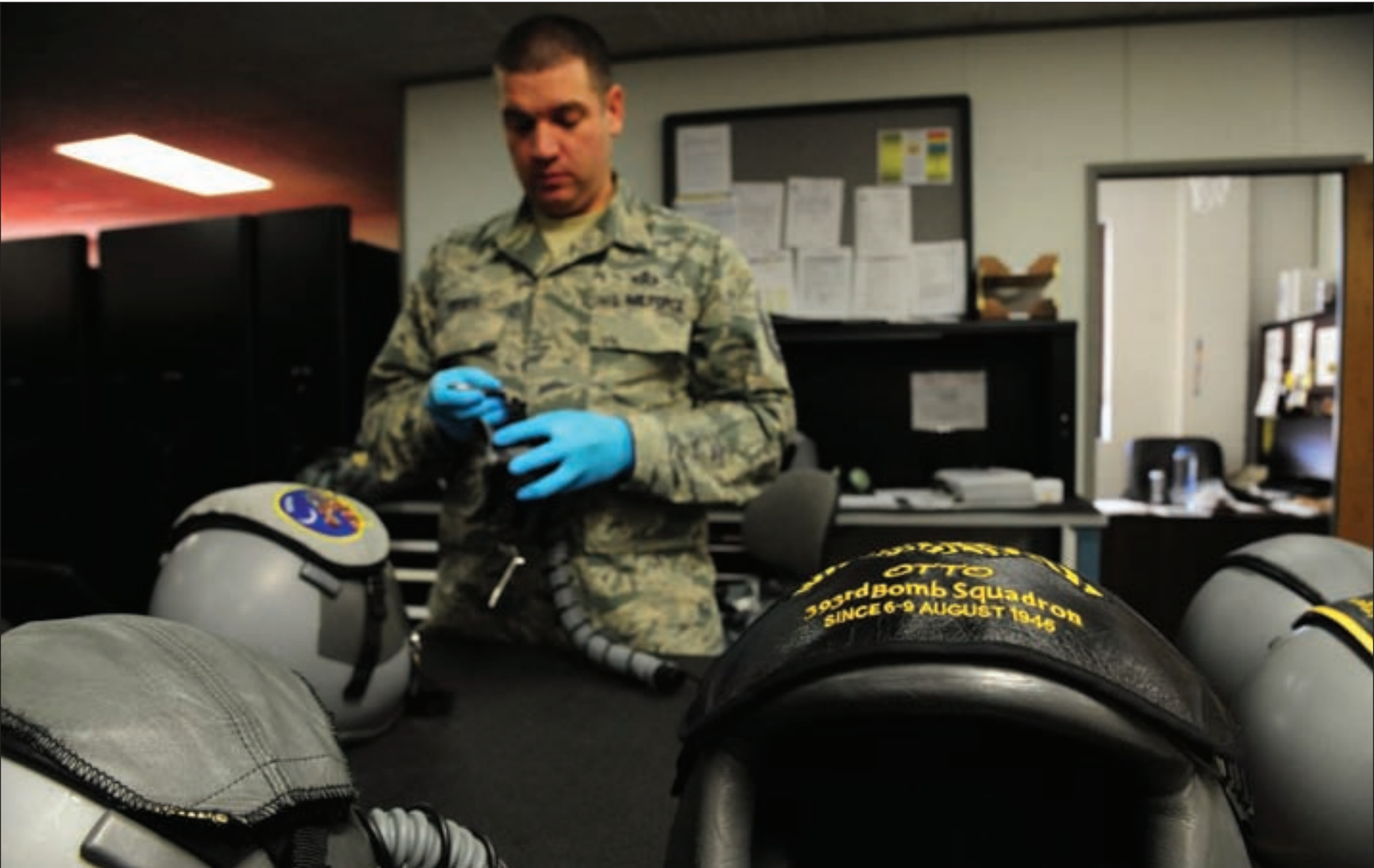
U.S. Air Force Master Sgt. Douglas Kraft, the 509th Operations Support Squadron aircrew flight equipment superintendent, performs a quality control inspection (QCI) on a Mask Breathing Unit-20/P at Whiteman Air Force Base, Mo., Dec. 1, 2015. A visual inspection of the oxygen mask is required to ensure the equipment is properly reassembled and functional.
