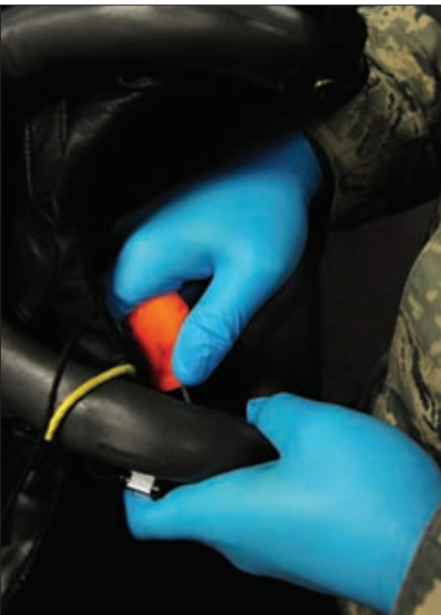
U.S. Air Force Master Sgt. Douglas Kraft, the 509th Operations Support Squadron aircrew flight equipment superintendent, inspects screws on a Mask Breathing Unit-Head Gear Unit 55P helmet during a quality control inspection at Whiteman Air Force Base, Mo., Dec. 1, 2015. The aircrew flight equipment personnel must make sure all screws on the helmets are tightened for the breathing components to function properly.
