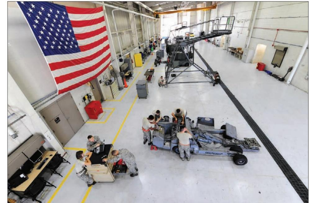
Airmen assigned to the aerospace ground equipment (AGE) shop perform maintenance on a bomb lift at Whiteman Air Force Base, Mo., Oct. 21, 2015. The mission of the AGE shop is to maintain and provide equipment for aircraft support.
