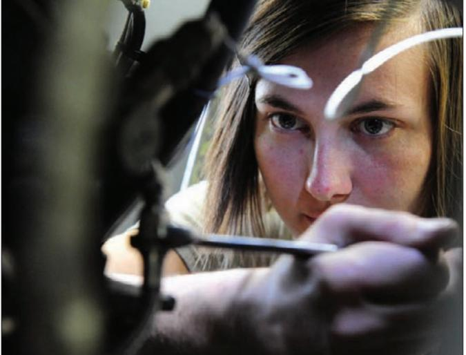
U.S. Air Force Airman 1st Class Melissa Jones, 509th Maintenance Squadron aerospace ground equipment apprentice, tightens a hydraulic line on a PD 501 air conditioner at Whiteman Air Force Base, Mo., Oct. 21, 2015. This procedure is done to prevent leaks from damaging the electrical components on the equipment.
