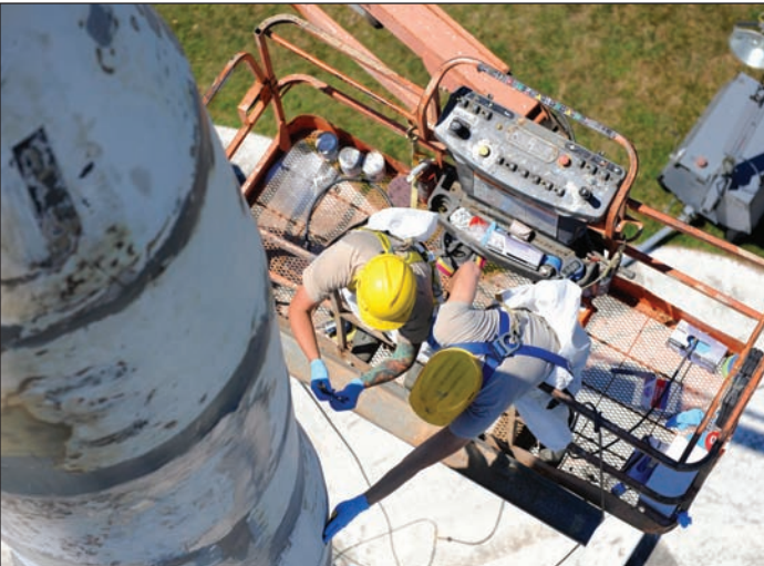
Members of the 509th Maintenance Squadron low observable shop perform maintenance on a Minuteman II Missile static display at Whiteman Air Force Base, Mo., Aug. 21, 2015. The missile was sanded, primed and then painted during the restoration process.
