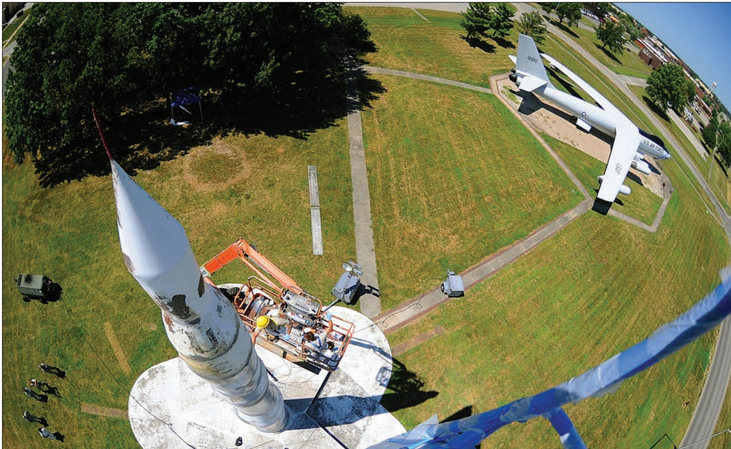
Members of the 509th Maintenance Squadron low observable shop perform maintenance on a Minuteman II Missile static display at Whiteman Air Force Base, Mo., Aug. 21, 2015. The missile was sanded, primed and then painted during the restoration process.
