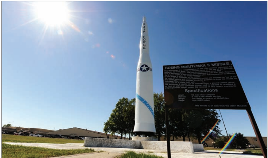
A Minuteman II Missile static display at Whiteman Air Force Base, Mo., was completely restored by the 509th Maintenance Squadron low observable shop recently. The missile was sanded, primed and then painted during the restoration process.
