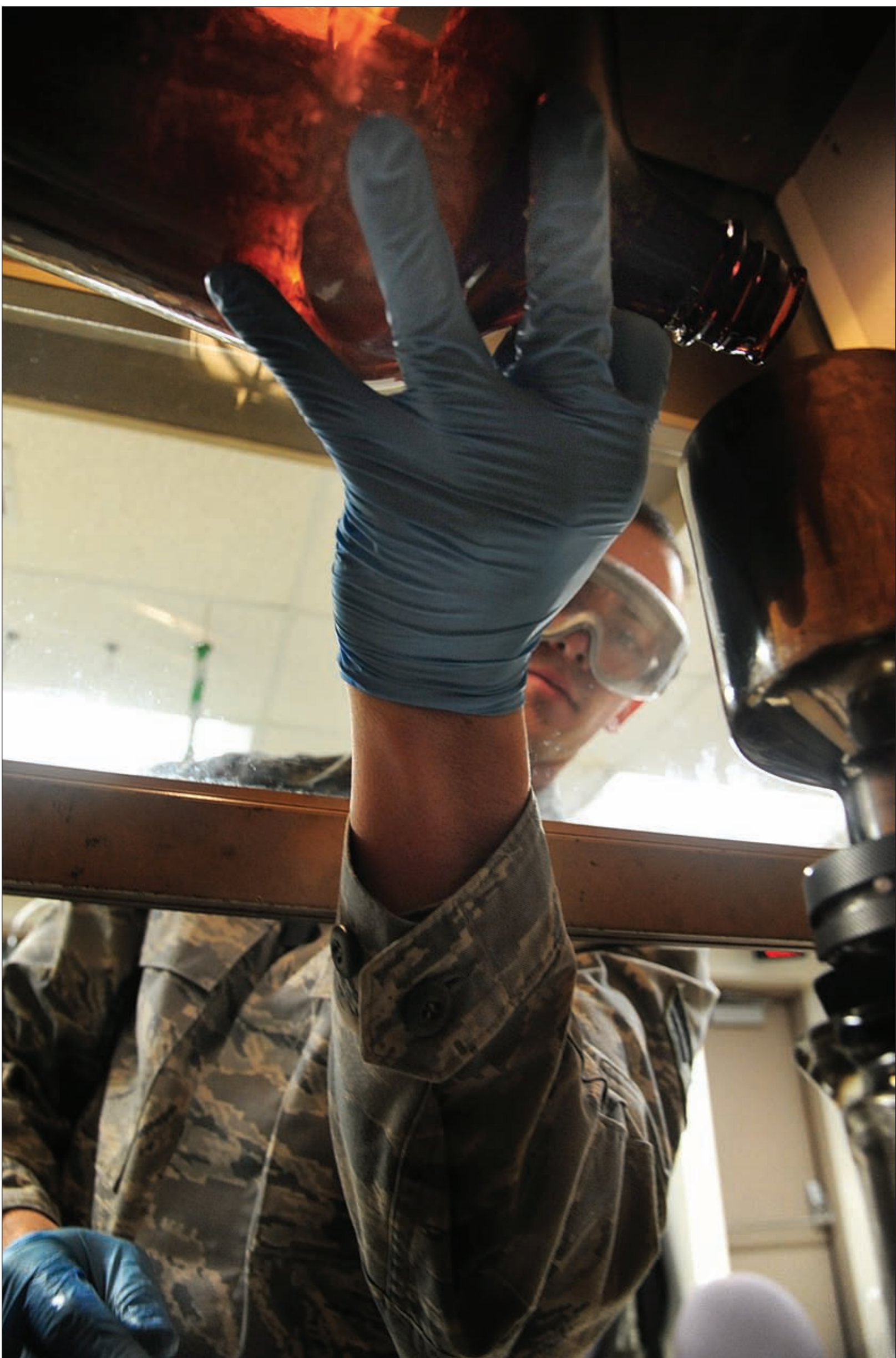
Senior Airman Christopher Croxton, 509th Logistics Readiness Squadron fuels lab technician, performs bottle method at Whiteman Air Force Base, Mo., April 22, 2015. This test provides a means to quantify the amount of articulate matter present in fuel.
