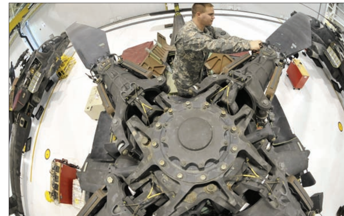
U.S. Air Force photo/Airman 1st Class Keenan Berry U.S. Army Spc. Todd Gann, 1-135th Attack/Reconnaissance Battalion aircraft maintainer, inspects the main rotor head of an AH-64 Apache at Whiteman Air Force Base, Mo., Jan. 9, 2014. Soldiers perform this inspection annually to ensure there are no signs of corrosion developing, which could cause malfunctions.
