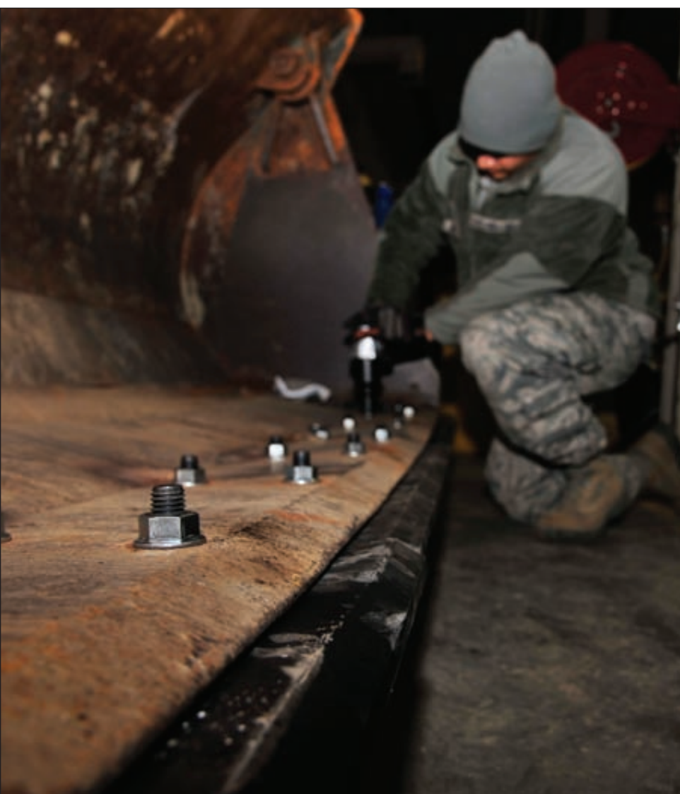
U.S. Air Force Staff Sgt. Nicholas Warkocz, 509th Civil Engineer Squadron supervisor, replaces loader bucket blades at Whiteman Air Force Base, Mo., Nov. 12, 2014. The blades wear down from constant usage, requiring them to be replaced.
