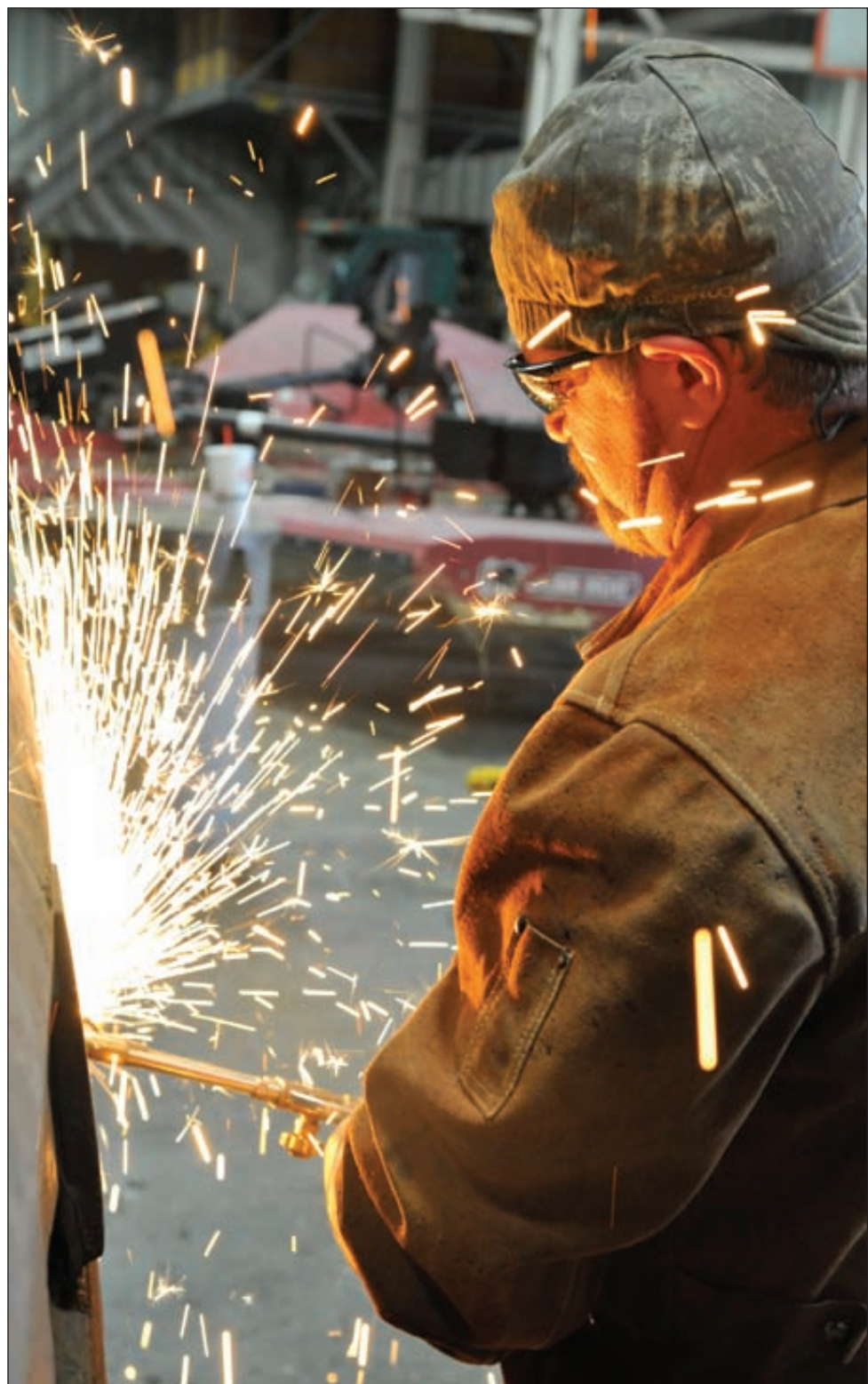
Bo Smith, 509th Civil Engineer Squadron tractor operator, welds the loader bucket at Whiteman Air Force Base, Mo., Nov. 4, 2014. This procedure is done to repair equipment damaged during operations.
