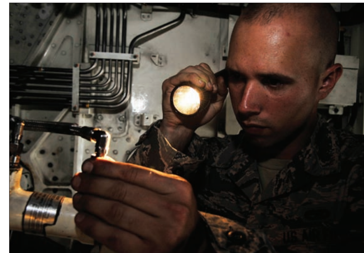
U.S. Air Force Staff Sgt. Clayton Walton, 509th Aircraft Maintenance Squadron crew chief, inspects a main lock gear actuator. The actuator must be inspected to ensure there is no fluid leaking or damage present.
