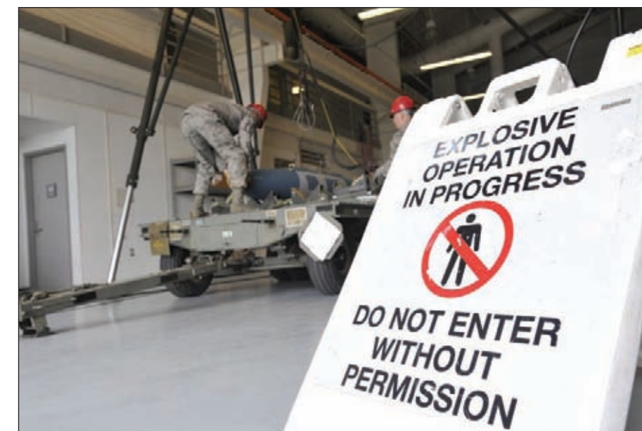
Airmen from the 509th Munitions Squadron conventional maintenance section use a munitions assembly conveyor to load munitions, using a device called the gantry, onto an MHU-110 trailer. The gantry is a sub-assembly of the MAC.
