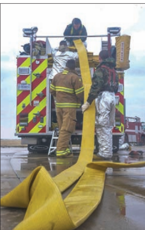
U.S. Air Force Civil Engineer Squadron firefighters load a hose onto a fire truck. A hook must be properly placed to ensure rapid deployment for the next emergency.
