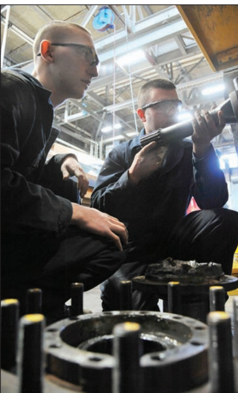
U.S. Air Force Air Force Airman 1st Class Cody Smith, 509th Logistics Readiness Squadron vehicle maintenance journeyman, left, and Staff Sgt. Kyle Bemis, 509th Logistics Readiness Squadron vehicle maintenance craftsman, remove broken axle shot at Whiteman Air Force Base, Mo., Feb. 21, 2014. The axle shot works with the differential to help the vehicle to move.
