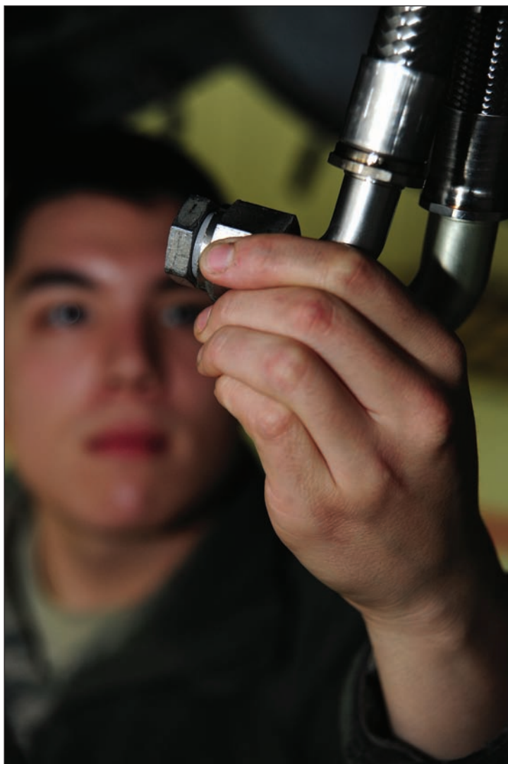
Airman 1st Class Cameron Wheatley, 442nd Fighter Wing Aircraft Maintenance Squadron aircraft armament technician, inspects the hydraulic lines of an A-10 Thunderbolt II gun. While performing the inspection Wheatley is looking for leaks and damage to the hydraulic line.
