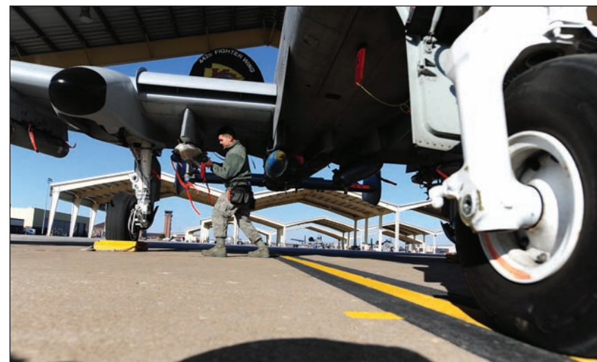
Airman 1st Class Cameron Wheatley, 442nd Fighter Wing Aircraft Maintenance Squadron aircraft armament technician, loads a BDU-33 training munition into the weapons array of an A-10 Thunderbolt II on the flightline. Not only does Wheatley load the weapons onto the aircraft, but he also performs operational checks to ensure the devices are functioning properly.
