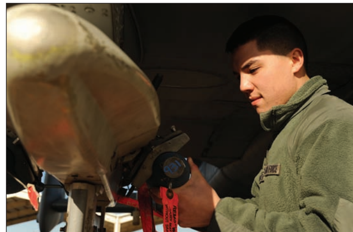
Airman 1st Class Cameron Wheatley, 442nd Fighter Wing Aircraft Maintenance Squadron aircraft armament technician, loads a BDU-33 training munition onto the weaponsrack of an A-10 Thunderbolt II. A-10 pilots drop weapons such as this one during training sorties as part of their target practice regimen.
