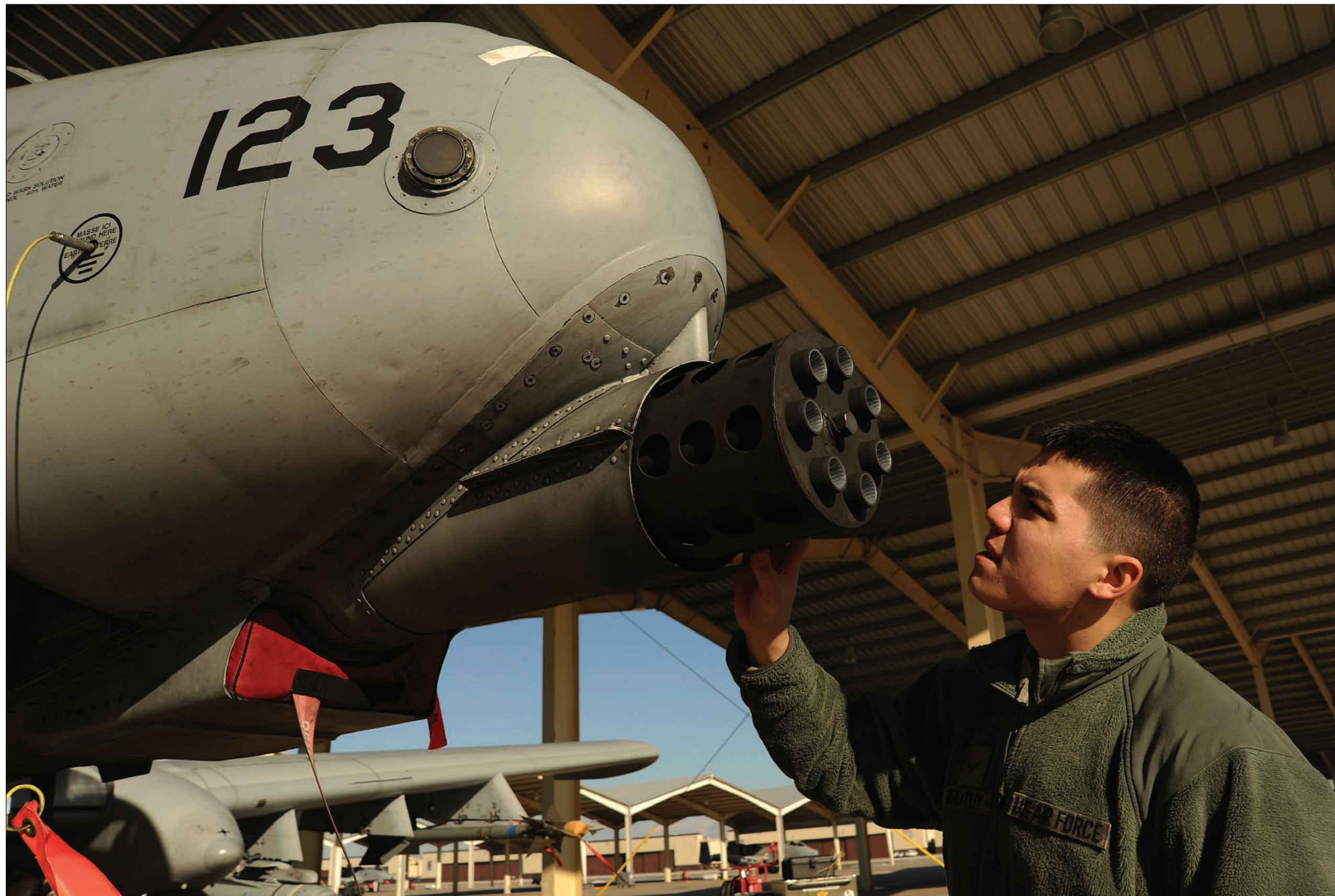
Airman 1st Class Cameron Wheatley, 442nd Fighter Wing Aircraft Maintenance Squadron aircraft armament technician, performs a 7-day gun-no-fire inspection on the Gatling gun of an A-10 Thunderbolt II at Whiteman Air Force Base, Mo., Dec. 17, 2013. The 30 mm seven-barrel gun allows pilots to accurately fire at ground targets.
