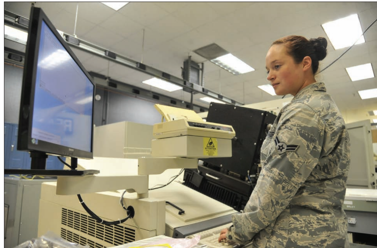
Airman 1st Class Samantha Bruton, 509th Maintenance Squadron avionics back shop team member, loads software for an actuator remote-terminal line-testing replaceable unit at Whiteman Air Force Base, Mo., July 25, 2013. Before the unit is used, it must be tested to ensure there are no system failures. If there are system failures, the avionics team will isolate the failed component from the test unit to prevent overall system failure.
