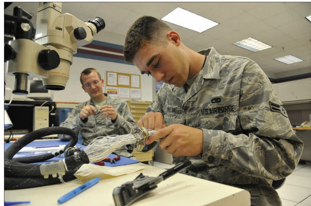
Airmen 1st Class James Lott and Michael Maluk, 509th Maintenance Squadron avionics back shop team members, remove and replace the back shell on a cannon plug at Whiteman Air Force Base, Mo., July 25, 2013. Stress over time, as well as normal wear, can cause back shells to break, requiring removal and replacing.
