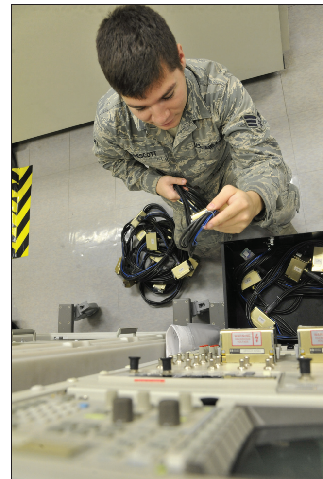
Senior Airman Christopher Prescott, 509th Maintenance Squadron avionics back shop team member, verifies inventory on portable calibration equipment at Whiteman Air Force Base, Mo., July 25, 2013. The avionics team performs semi-annual inspections to ensure no equipment is missing or damaged, and they recalibrate equipment every 180 days to verify the test station's serviceability.
