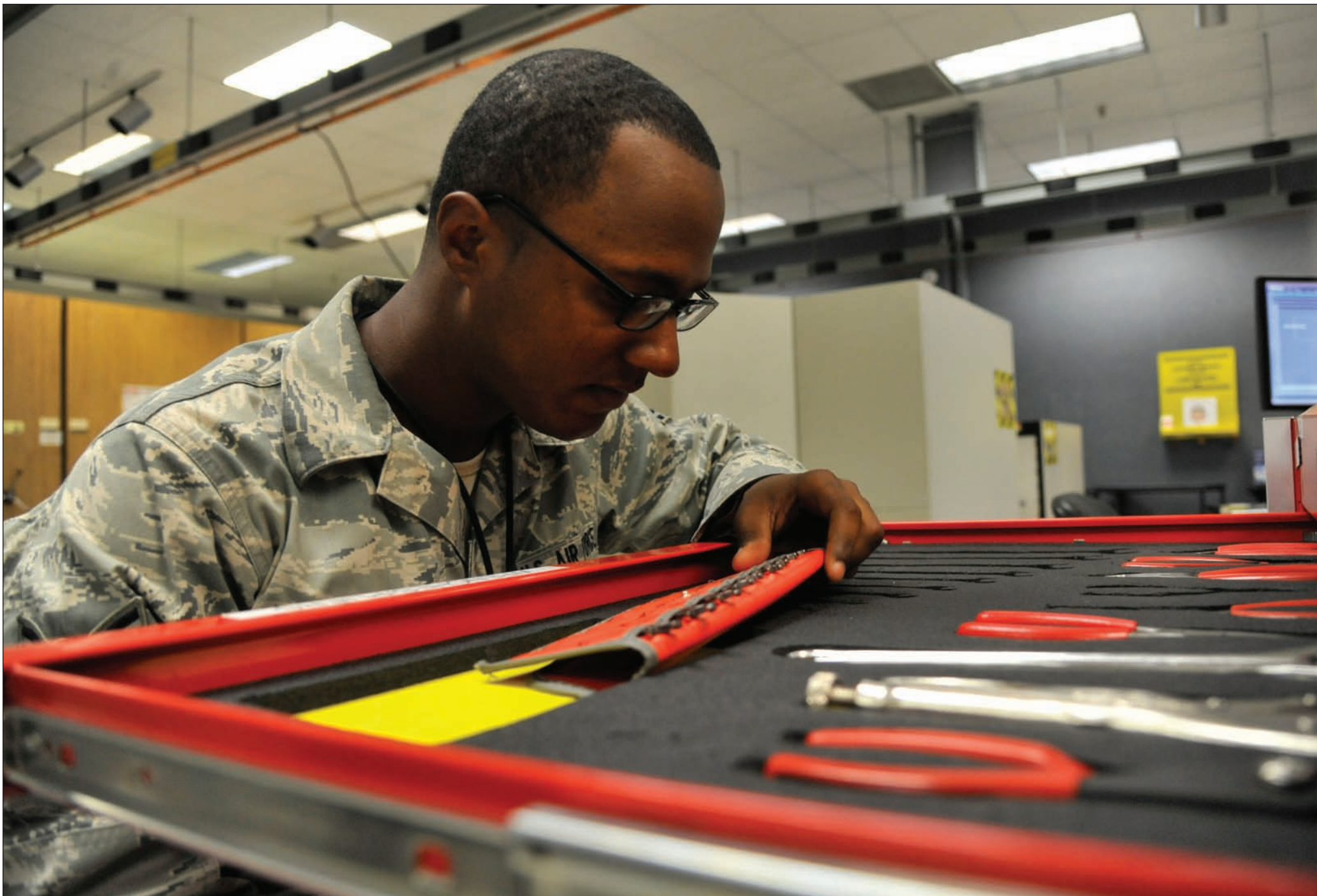
Airman 1st Class Michael Touchette, 509th Maintenance Squadron avionics back shop team member, inspects a tap and die set at Whiteman Air Force Base, Mo., July 25, 2013. The tap and die set must be inspected to ensure there are no damaged or missing tools. These tools are used to re-thread screws on line replaceable units and to prevent personality modules threads from stripping.
