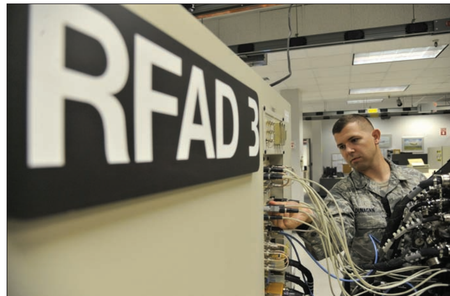
Airman 1st Class Samantha Bruton, 509th Maintenance Squadron avionics back shop team member, loads software for an actuator remote-terminal line-testing replaceable unit at Whiteman Air Force Base, Mo., July 25, 2013. Before the unit is used, it must be tested to ensure there are no system failures. If there are system failures, the avionics team will isolate the failed component from the test unit to prevent overall system failure.
