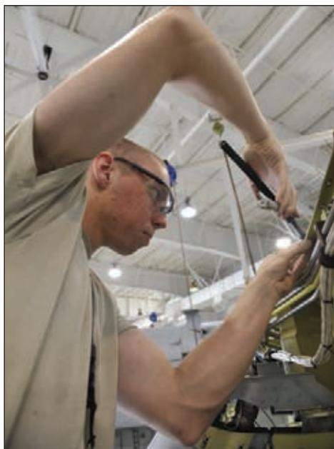
Airman 1st Class Lawrence Bowman, Detachment 303 Aircraft Maintenance Squadron structural maintenance apprentice, removes nut plates on an A-10 Thunderbolt II at Whiteman Air Force Base, Mo. July 1, 2013. Rivets are installed to hold the nut plates and keep the leading wing from tearing off.
