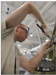
Airman 1st Class Lawerence Bowman, Detachment 303 Aircraft Maintenance Squadron structural maintenance apprentice, removes nut plates on an A-10 Thunderbolt II at Whiteman Air Force Base, Mo. July 1, 2013. Rivets are installed to hold the nut plates and keep the leading wing from tearing off.
