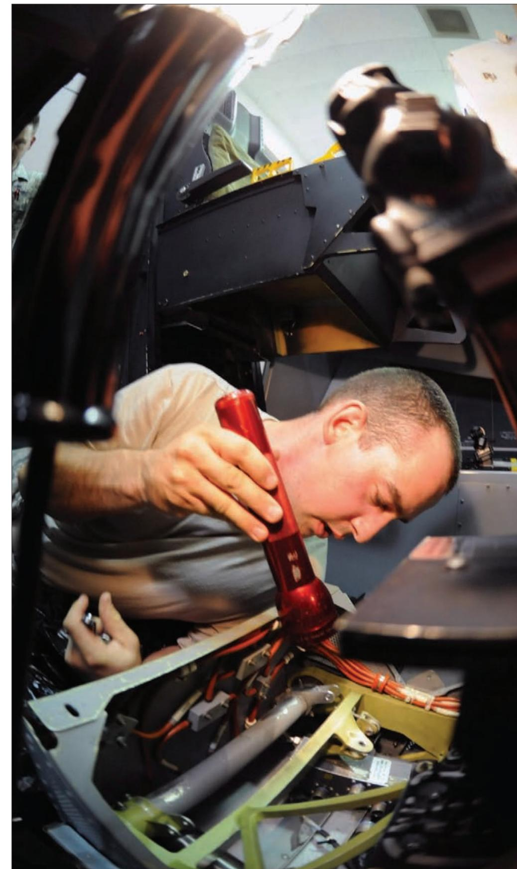
Senior Airman John T. Eckardt, 372nd Training Squadron, Det. 6, B-2 Spirit instruments and flight controls instructor, determines the best way to fix a pitch torque tube and pitch positioning sensor assembly at Whiteman Air Force Base, Mo., June 12, 2013. One of the many challenges avionics mechanics face is limited room to maneuver their bodies and hands inside the panels.
