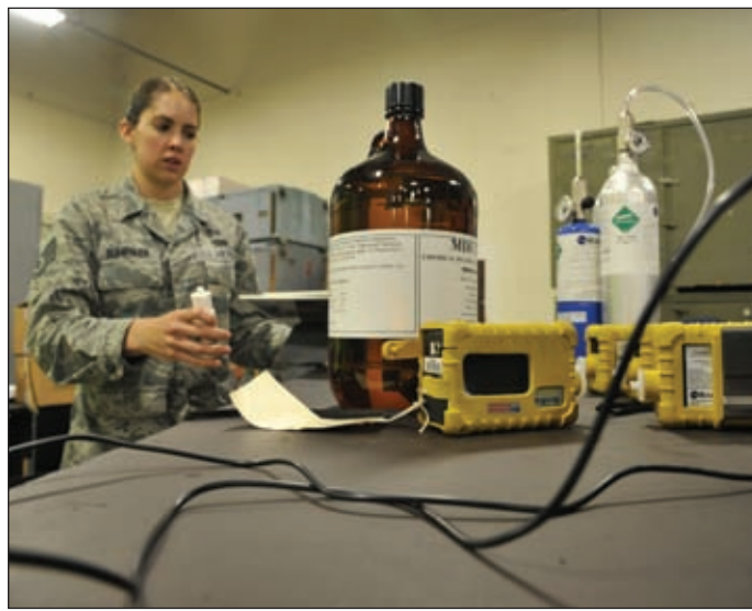
Staff Sgt. Rebecca Buhrman, 509th Civil Engineer Squadron NCO in charge of emergency management logistics, and Airman 1st Class Alfredo Guzman, 509th CES journeyman, set up the hazardous material identifier (HAZMAT ID) at Whiteman Air Force Base, Mo., May 22, 2013. Airmen use the HAZMAT ID to detect chemicals and biological agents, and provides readouts of tested material, showing whether contamination is present or not.
