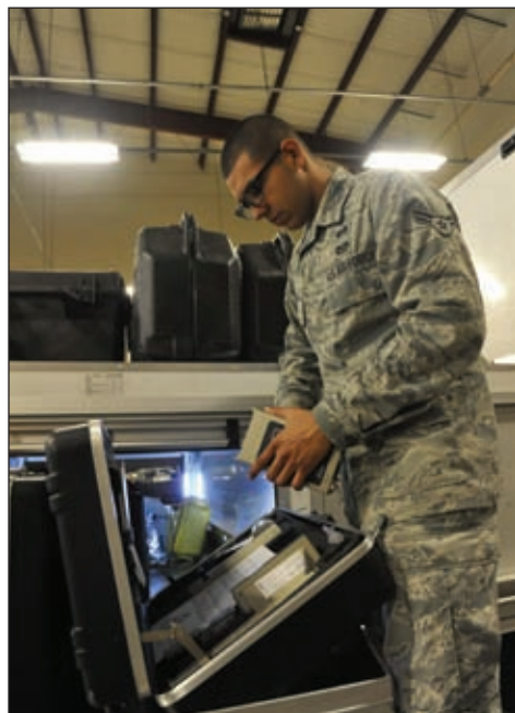
Airman 1st Class Alfredo Guzman, 509th Civil Engineer Squadron journeyman, performs an operation check on the ADM-300 at Whiteman Air Force Base, Mo., May 22, 2013. This equipment is used to measure levels of radiation, and is inspected every week to ensure proper functioning.
