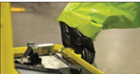
Airman 1st Class Brandon Stone, 509th Civil Engineer Squadron apprentice, uses a spectrometer to analyze white powder during training at Whiteman Air Force Base, Mo., May 22, 2013. The spectrometer is used to identify liquids and powders from suspicious packages that may contain explosives.
