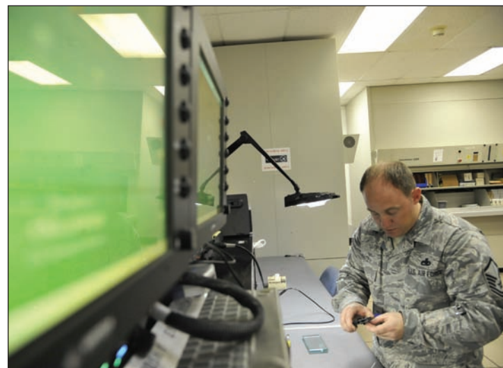
Master Sgt. Michael White, 509th Maintenance Operations Squadron B-2 Spirit computer-aided design manager, crimps a pin on the adaptable communications suite keyboard at Whiteman Air Force Base, Mo., May 15, 2013. Research engineers provide repairs for ACS keyboards by making the wires more durable.
