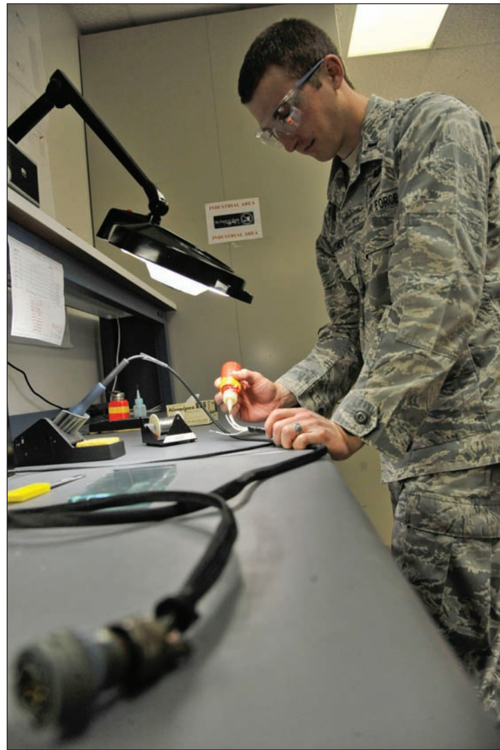
1st Lt. Andrew Klausner, 509th Maintenance Operations Squadron flight commander, solders wiring for the adaptable communications suite keyboard at Whiteman Air Force Base, Mo., May 15, 2013. Soldering makes wires more rigid, preventing them from crimping and presenting a maintenance problem.
