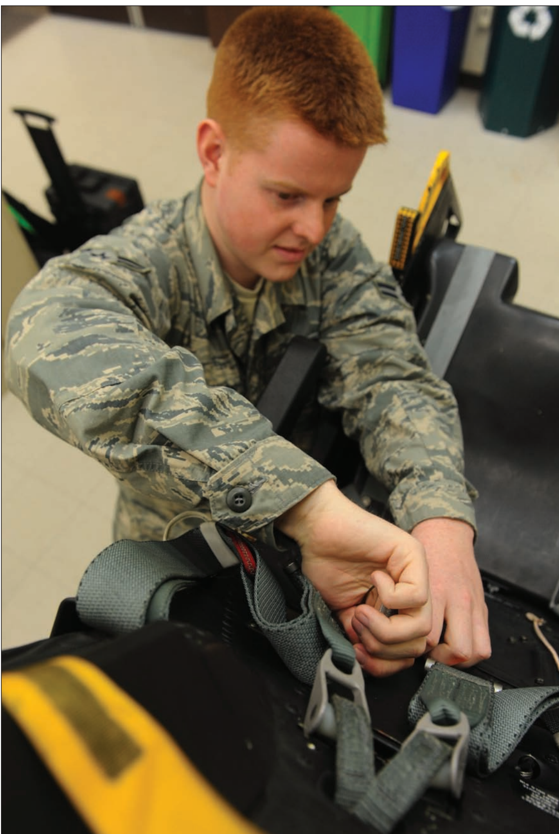
Airman 1st Class Christopher Amsel, 509th Maintenance Squadron egress systems journeyman, inspects a retaining pin on a training ejection seat parachute at Whiteman Air Force Base, Mo., March 19, 2013. The egress shops work schedule varies depending on flight operations each week.
