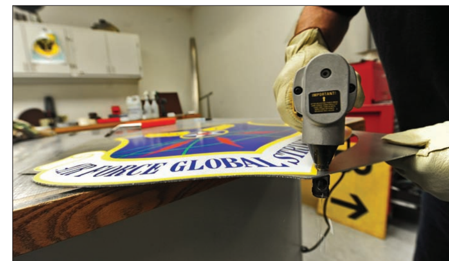
Bernard Jones, 509th Civil Engineer Squadron sign maker, uses a nibbler to cut away excess aluminum from a Global Strike Command insignia at Whiteman Air Force Base, Mo., March 11, 2013. MAJCOM signs help show visitors and newcomers the command's ownership of the installation.
