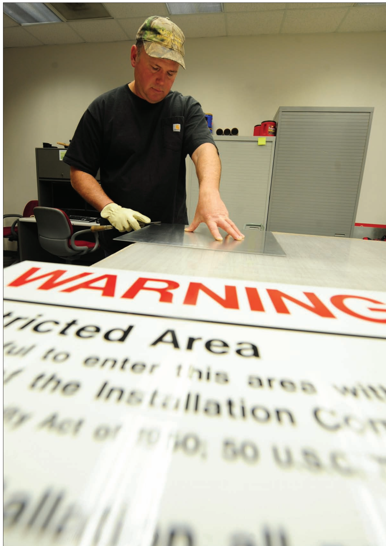
Bernard Jones, 509th Civil Engineer Squadron sign maker, prepares a restricted area sign for vinyl coating at Whiteman Air Force Base, Mo., March 11, 2013. The vinyl coating acts as an adhesive that enables personnel to attach the banner to the aluminum sign frame.
