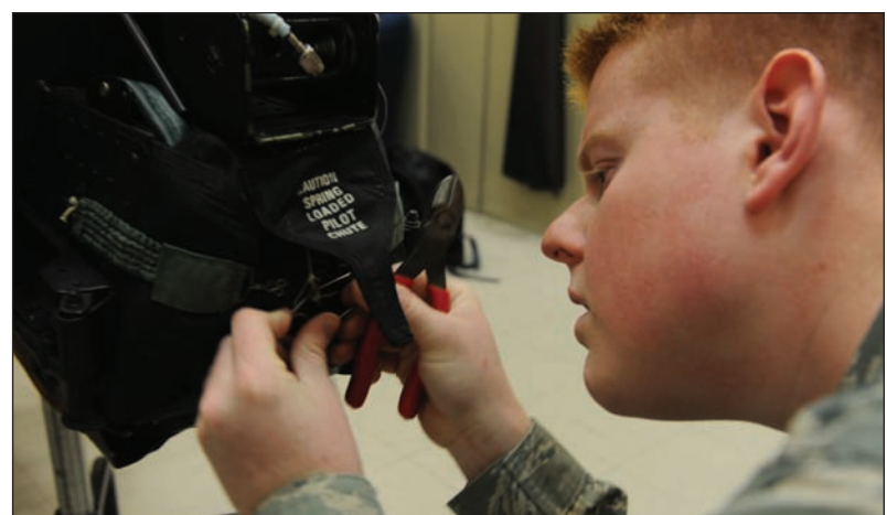
Airman 1st Class Christopher Amsel, 509th Maintenance Squadron egress systems journeyman, inspects a retaining pin on a training ejection seat parachute at Whiteman Air Force Base, Mo., March 19, 2013. The egress shops work schedule varies depending on flight operations each week.
