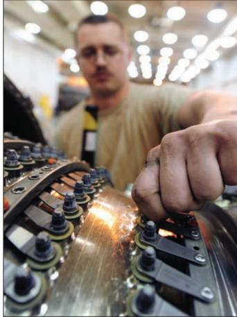
Senior Airman Brady Dell, 509th Maintenance Squadron aerospace propulsion journeyman, checks the actuator of a B-2 Spirit engine for tightness, Feb. 13. One loose bolt could destroy the multi-million dollar engine during flight and possibly cause a B-2 to crash.
