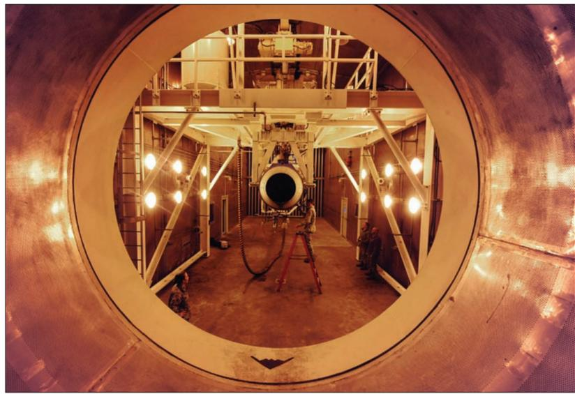
Airman 1st Class Lester Popham, 509th Maintenance Squadron aerospace propulsion apprentice, inspects the exhaust of a B-2 Spirit engine for foreign object debris and oil in the test cell, Feb. 13. A thorough inspection helps mechanics find items that might destroy the engine or the test cell.
