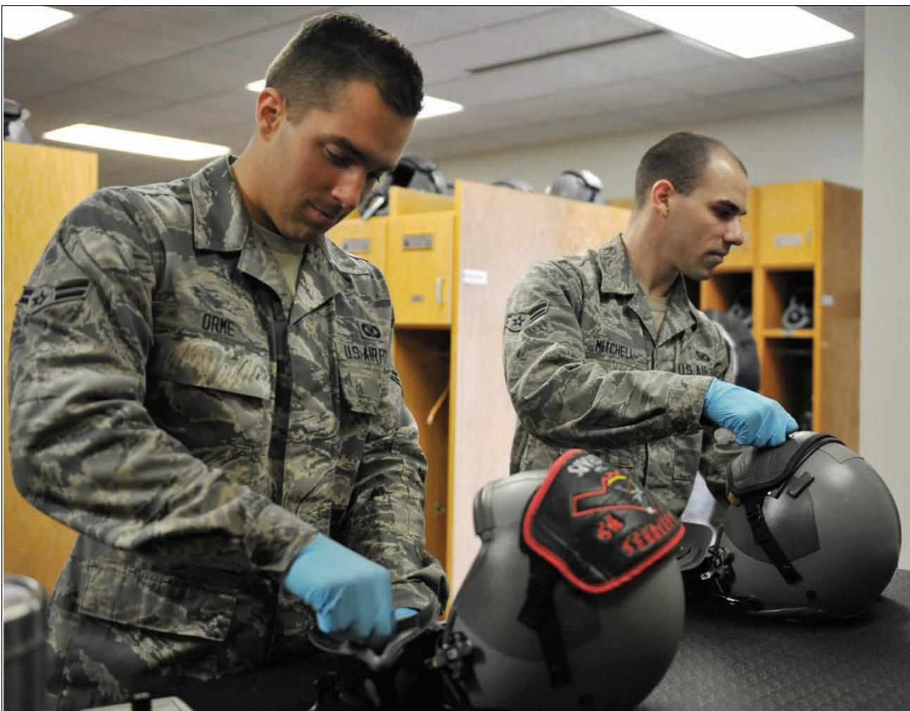
Airman 1st Class Devin Orme and Airman 1st Class Eric Mitchell, 509th Operations Support Squadron aircrew flight equipment journeymen, clean oxygen masks, Jan. 18. Aircrew flight equipment specialists inspect, maintain and adjust life support and survival gear for flight-crew members assigned to Whiteman AFB.
