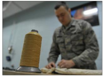
Airman 1st Class Chris Lineberry, 509th Operations Support Squadron aircrew flight equipment journeyman, checks the pull-test on the restrictor lanyard, Jan. 18. Airmen conduct pull-tests to ensure correct opening sequence on a parachute in case it were to deploy.
