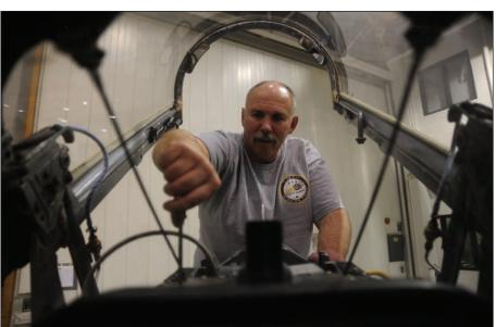
Russ Cass, M1 Support Services aircraft mechanic, checks the tightness of a screw on an ejection seat in a T-38 Talon, Jan. 24. The ejection seat is rocketpowered to allow pilots to escape the aircraft in case of an emergency.
