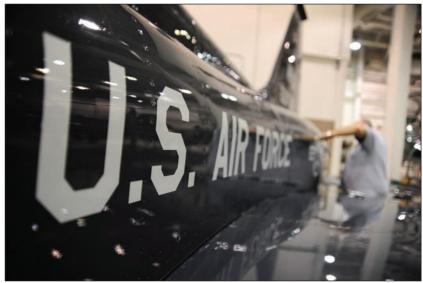
Russ Cass, M1 Support Services aircraft mechanic, secures an access panel for a hydraulic reservoir on a T-38 Talon, Jan. 24. These panels enable mechanics to more easily access the aircraft and perform repairs on various components.
