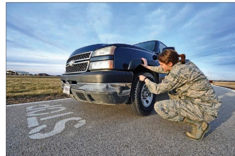
Airman 1st Class Heather Hall, 509th Operations Support Squadron airfield management coordinator, performs a check for foreign object debris before dispersing a bird threat, Jan. 9. FOD checks help keep aircraft free of small fragments that can potentially cause damage to aircraft.
