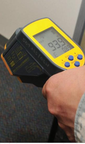
Tech. Sgt. Ryan Watts, 509th Operations Support Squadron, demonstrates an infrared temperature gun during his shift Sept. 13. The Weather Flight uses the device to take temperature readings and is primarily used in the winter to determine the rate at which snow melts.
