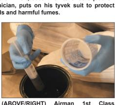
Mathew Wert, 509th Maintenance Squadron low observable technician, measures paint for the B-2 Spirit coating. The LO section maintains the stealth capabilities of the B-2 by repairing the LO coating and internal and external structural hardware.
