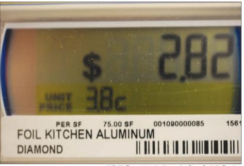
An electronic shelf display shows price rates at the commissary here Oct. 7. The new displays use infrared technology connected to computer servers to automatically update product pricing providing accurate information without the need of manual labor.
