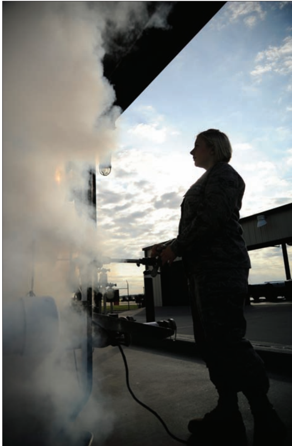
Senior Airman Deserea Sandquist, 509th Logistics Readiness fixed-facilities fuels technician, bleeds an oxygen tank here Aug. 31 to release pressure and ensure air quality.
