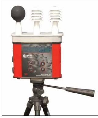
U.S. Air Force photo illustration/ Tech. Sgt. Kent Kagarise The wet bulb is a device used by the 442nd FW Bioenvironmental shop to determine the work schedule for military members. The 442nd Bioenvironmental shop is part of the 442nd FW Medical Squadron, of the 442nd Fighter Wing, an A-10 Thunderbolt II Air Force Reserve unit at Whiteman Air Force Base, Mo.
