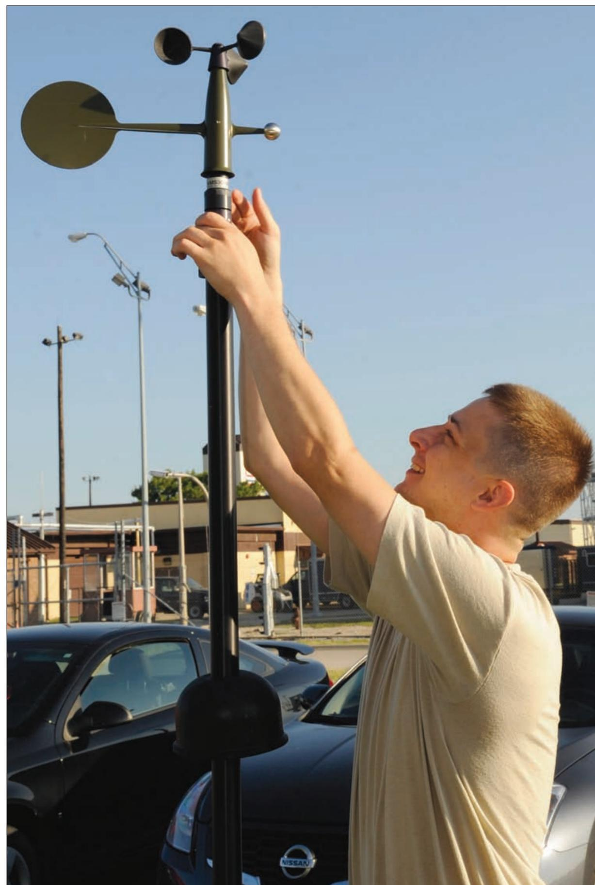
Staff Sgt. Ryan Watts, 509th Operation Support Squadron weather training NCO in charge, sets up the tactical meteorological observing systems to perform routine maintenance here July 20. The suite of automatic tactical weather sensors provides an automated collection of weather elements in deployed environments.
