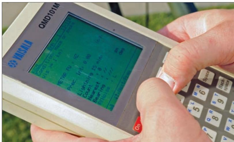
Staff Sgt. Ryan Watts, 509th Operation Support Squadron weather training NCO in charge, performs a routine maintenance inspection on tactical meteorological observing systems here July 20. The system takes environmental weather conditions such as wind, rain, lightening, present temperature, dew point, humidity and present weather.
