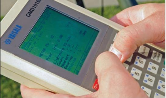
Staff Sgt. Ryan Watts, 509th Operation Support Squadron weather training NCO in charge, performs a routine maintenance inspection on tactical meteorological observing systems here July 20. The system takes environmental weather conditions such as wind, rain, lightening, present temperature, dew point, humidity and present weather.
