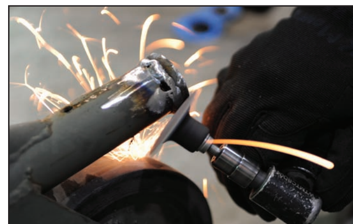
(Left) Staff Sgt. Kevin Monfreda, 509th Maintenance Squadron aircraft metals technologist, grinds down paint and rust from an existing weld ensuring it is not compromised in preparation for welding a new section for a C-1 maintenance stand, Nov. 1. (Below left) An Airman from the 131st Maintenance Squadron holds an Air Force Global Strike Command emblem
