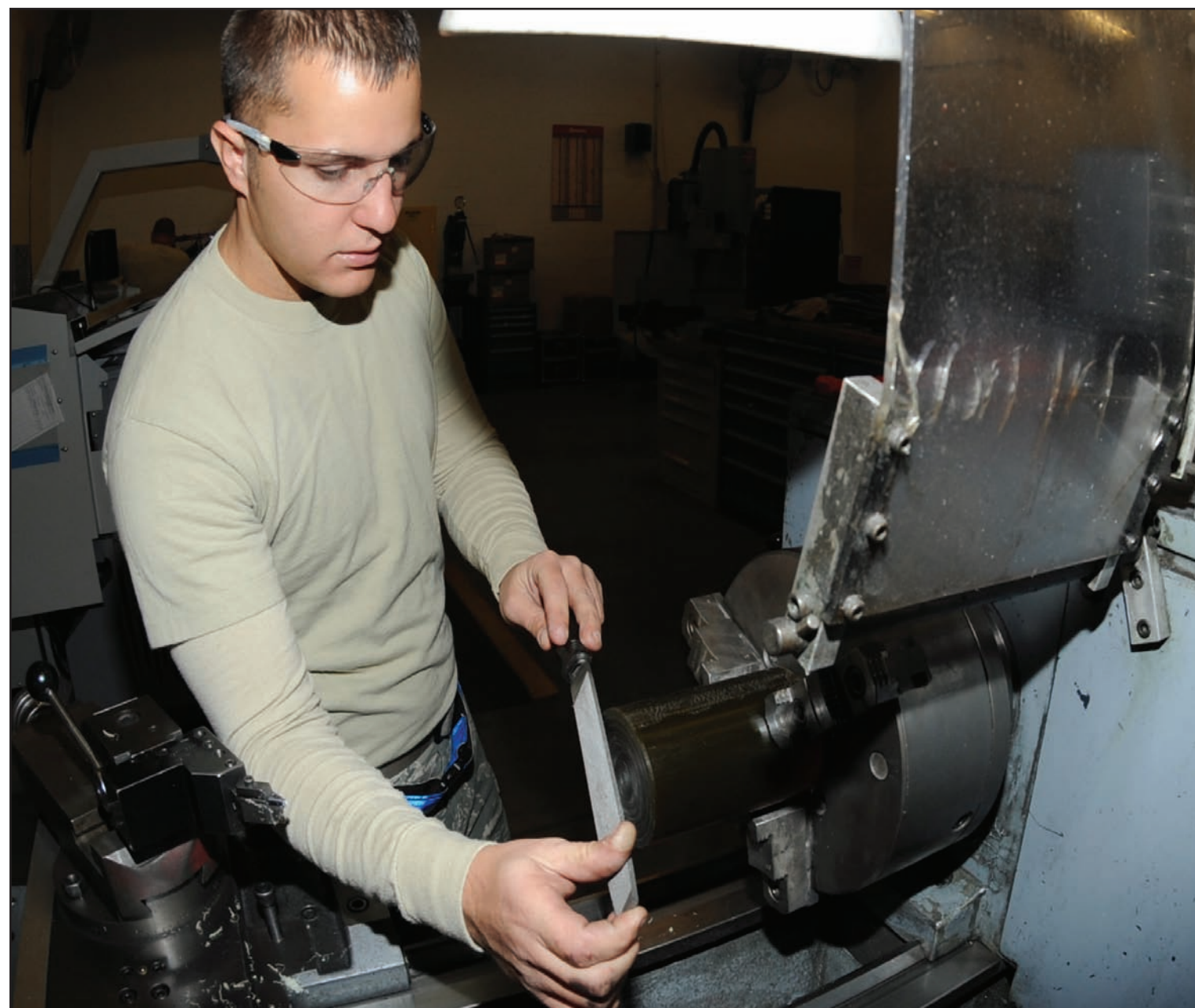
(Left) Senior Airman Steven Edwards, 509th Maintenance Squadron metals technology journeyman, cleans up the edges of a rudder actuator collar with a rasp on the machining lath, Nov. 3. The rudder actuator collar will be used by maintenance members when working on the rudder assembly to safely allow them to prop the rudder up without injury. (Below) The machining mill is used to remove excess material from the core of a rudder actuator collar.
