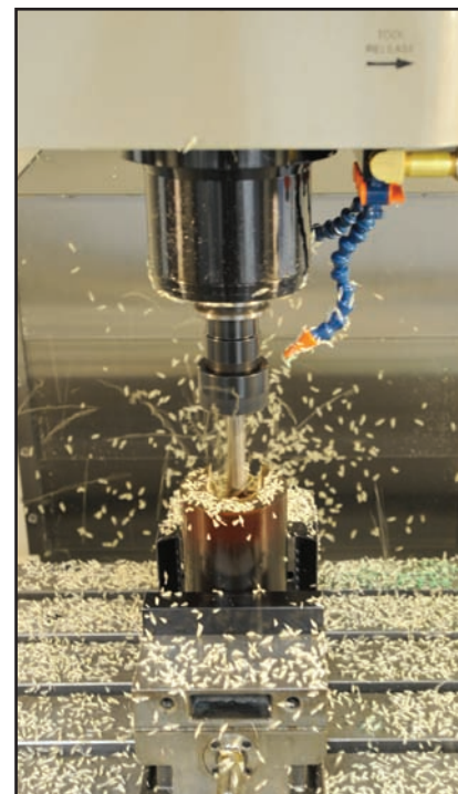
(Left) Senior Airman Steven Edwards, 509th Maintenance Squadron metals technology journeyman, cleans up the edges of a rudder actuator collar with a rasp on the machining lath, Nov. 3. The rudder actuator collar will be used by maintenance members when working on the rudder assembly to safely allow them to prop the rudder up without injury. (Below) The machining mill is used to remove excess material from the core of a rudder actuator collar.
