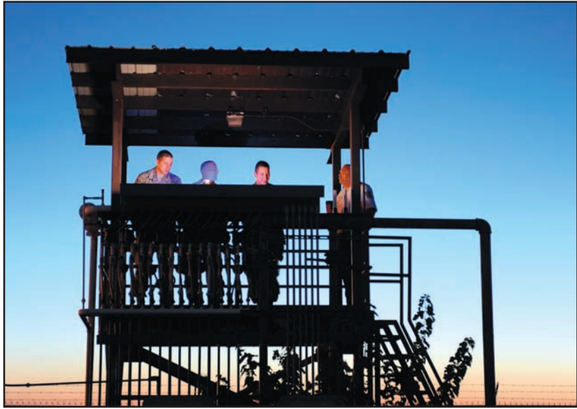
Left: Whiteman firefighters from the 509th Civil Engineer Squadron, operate the fire pit from a control booth, Aug. 23. The control booth regulates and directs the propane gas that fuels the fire, allowing them to choose between engine, wing and cockpit fires so Airmen can train in all three areas.
