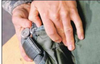
Left: Tech. Sgt. Michael Cole 393rd Aircrew Flight Equipment NCO in-charge inspects the torso harness used in the B-2 ejection seat. The TO gives step-by-step procedures on inspecting safety equipment.
