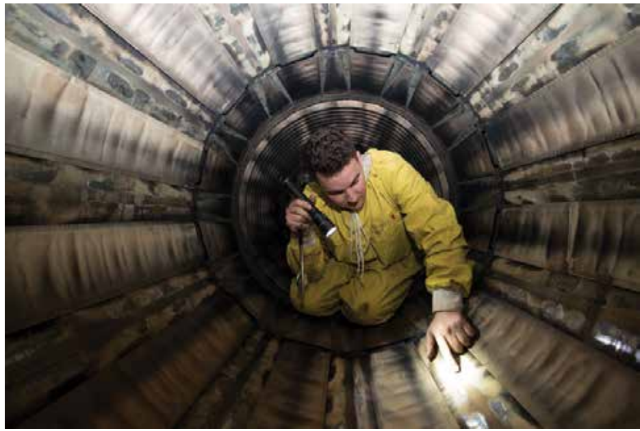
Staff Sgt. Adam Bowen, 55th Expeditionary Fighter Squadron phase floor chief, inspects an F-16C Fighting Falcon's engine exhaust for damage at an undisclosed location in Southwest Asia, Feb. 10, 2019. In addition to fulfilling all required actions identified by the flightline maintainers, phase personnel also perform in-depth nose-to-tail inspections of every jet that comes through their shop. (U.S. Air Force photo by Tech. Sgt. Clinton Atkins)
