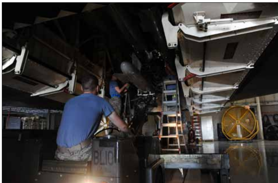
U.S. Air Force Airman 1st Class Christopher Glassen, a 13th Aircraft Maintenance Unit weapons load crew member, drives a B61-7 training munition into a weapons load trainer using a MHU-83 D/E jammer at Whiteman Air Force Base, Mo., July 15, 2016. Every three months, the most efficient crew from each aircraft maintenance unit within the 509th and 131st Aircraft Maintenance Squadrons competes for the Load Crew of the Quarter award.
