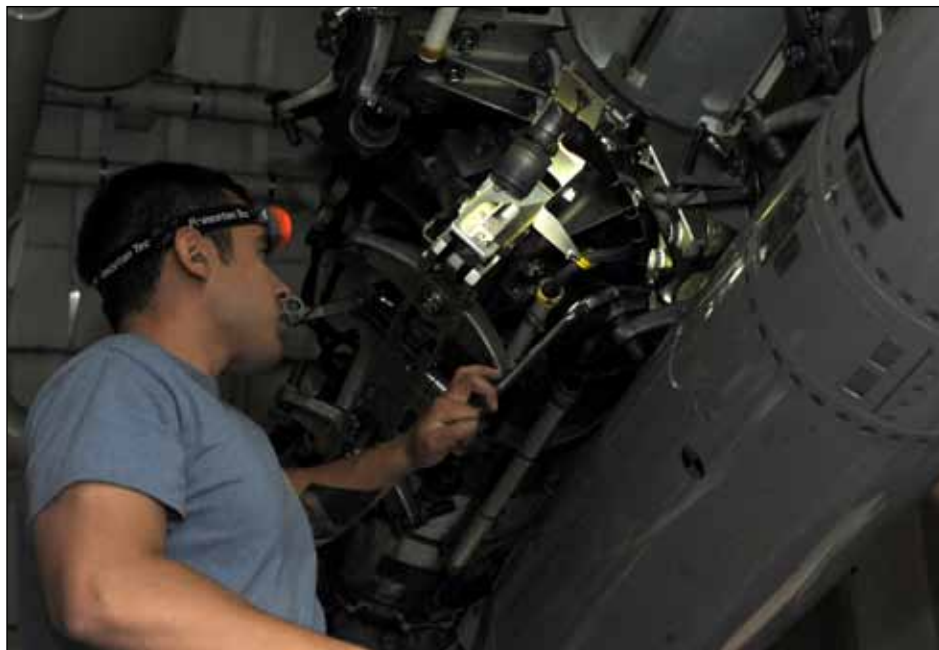
U.S. Air Force Staff Sgt. Brenton Swift, a 13th Aircraft Maintenance Unit (AMU) weapons load crew chief, secures a B61-7 training munition into a weapon load trainer's bomb rack during a Load Crew of the Quarter competition at Whiteman Air Force Base, Mo., July 15, 2016. The B-2 Spirit weapons load trainer is a model that allows weapons loaders to practice loading more frequently and when a B-2 aircraft isn't available.
