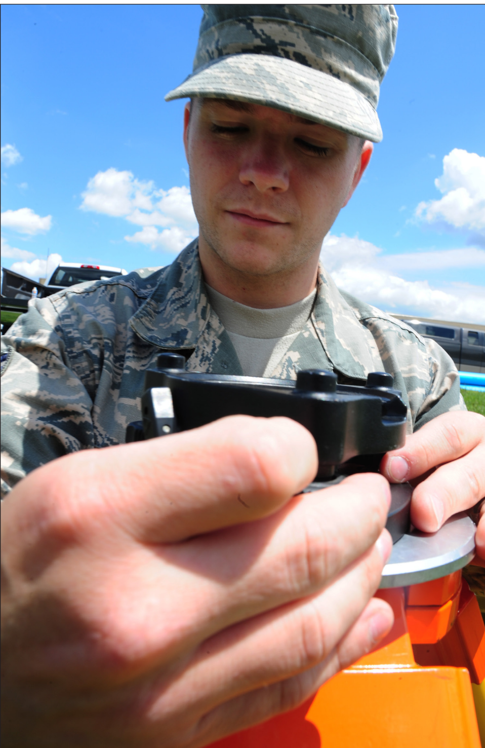
U.S. Air Force Airman 1st Class Nicholas Bara, a 509th Civil Engineer Squadron engineering technician, sets up a total station at Whiteman Air Force Base, Mo., May 18, 2016. Total stations are electronic optical instruments used to give precise angles and distances for a building's foundation.
