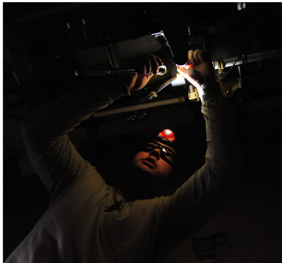
U.S. Air Force Senior Airman Brandon Anderson, a 393d Aircraft Maintenance Unit (AMU) load crew member, prepares the bomb rack sway pads prior to loading an AGM-158 Joint Air-to-Surface Standoff Missile during a weapons load competition at Whiteman Air Force Base, Mo., April 27, 2016. Total Force Airmen from the 131st and 393d AMU competed in the competition to test the crews' ability to load weapons in a timely manner.
