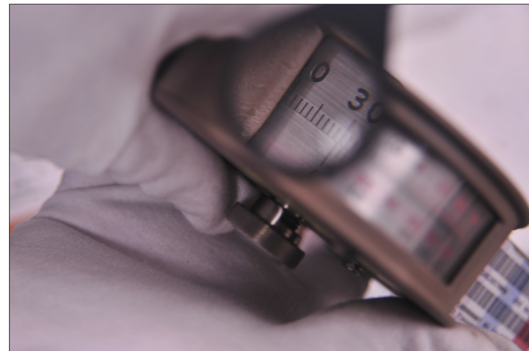
U.S. Air Force photo/Senior Airman Jovan Banks Marc Morris, a precision measurement equipment laboratory (PMEL) technician assigned to the 509th Maintenance Squadron, holds a clinometer during equipment testing at Whiteman Air Force Base, Mo., May 4, 2016. PMEL technicians use clinometers to measure slopes and angles when doing equipment testing.
