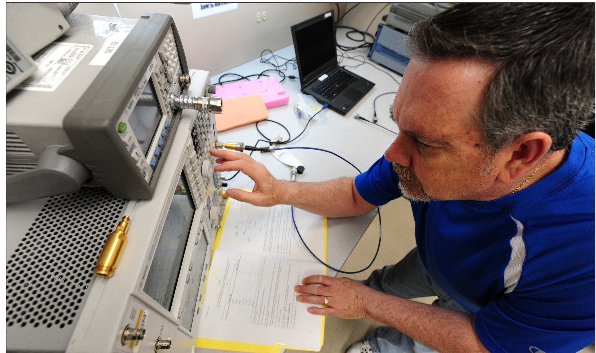
U.S. Air Force photo/Airman 1st Class Keenan Berry Craig Mayeux, a 509th Maintenance Squadron precision measurement equipment laboratory technician, initiates a test on an audio analyzer at Whiteman Air Force Base, Mo., May 4, 2016. An audio analyzer is a test and measurement instrument used to quantify the audio performance of electronic and electro-acoustical devices.
