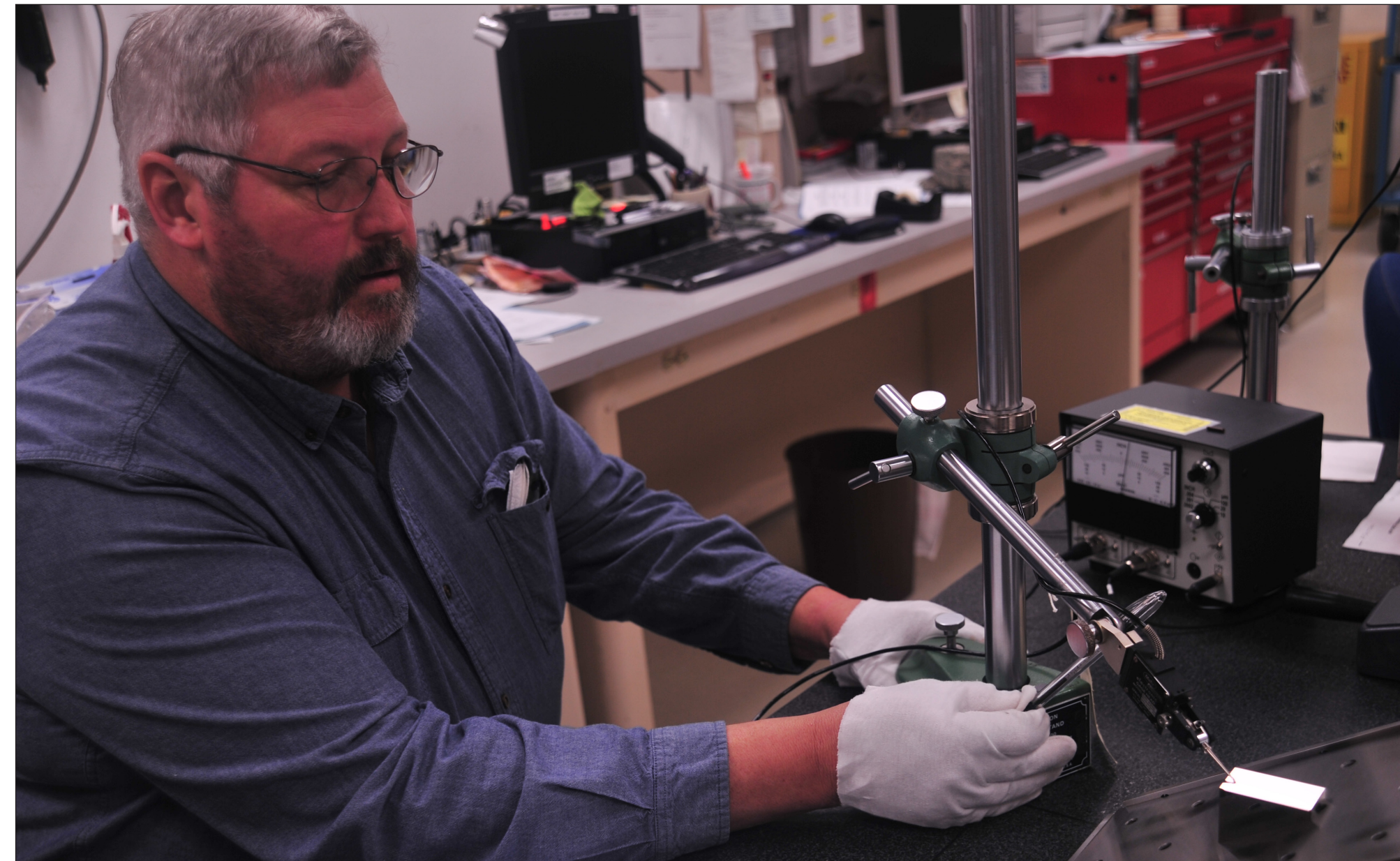
U.S. Air Force photo/Senior Airman Jovan Banks Marc Morris, a precision measurement equipment laboratory (PMEL) technician assigned to the 509th Maintenance Squadron, adjusts a precision-angle block before measuring test equipment at Whiteman Air Force Base, Mo., May 4, 2016. The equipment tested by PMEL technicians is used by various squadrons throughout Whiteman.
