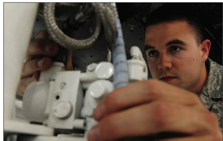
U.S. Air Force Airman Stephen Shaff, an electrical environment systems specialist from the 358th Fighter Squadron, inspects cannon plugs on an A-10 Thunderbolt II's nosewheel steering harness at Whiteman Air Force Base, Feb. 18, 2016. This procedure is done to ensure the cannon plugs are in good condition and there is no damage. If the plugs are damaged, they could cause severe damage to the aircraft's wheel component.
