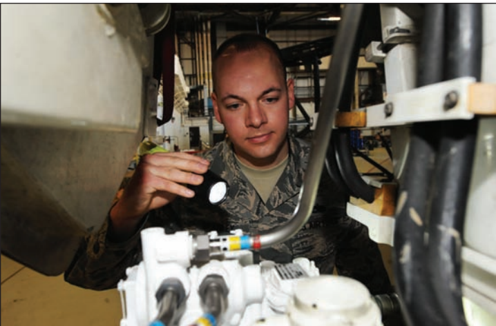
U.S. Air Force Tech. Sgt. Aaron Bradley, a 393d Aircraft Maintenance Unit specialist section chief, inspects the hydraulic lines of a B-2 Spirit at Whiteman Air Force Base, Mo., Feb. 18, 2016. The inspection of the 4,000 psi hydraulic system tests operation of the B-2 flight controls, landing gear, brakes, steering and weapon systems.
