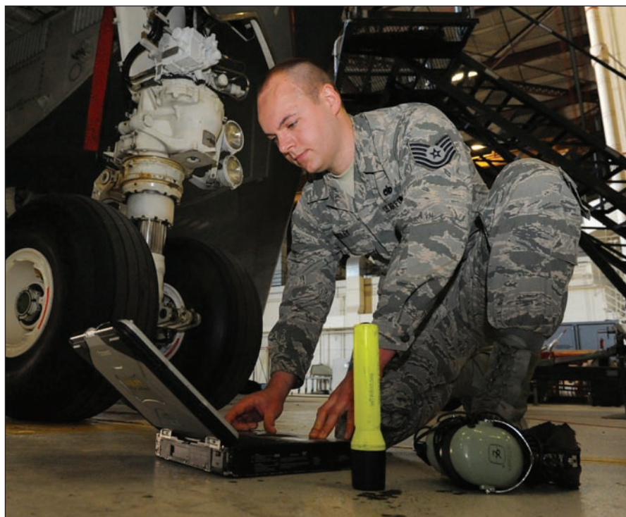
U.S. Air Force Tech Sgt. Aaron Bradley, a 393d Aircraft Maintenance Unit specialist section chief, uses a socket wrench to adjust the front landing gear of a B-2 Spirit at Whiteman Air Force Base, Mo., Feb. 18, 2016. When needed, Bradley wears a headset to communicate with a second member in the cockpit—who applies hydraulic pressure. This method allows the crew to adjust the steering of the front landing gear without actually turning the wheel, which prevents wear on the tires.
