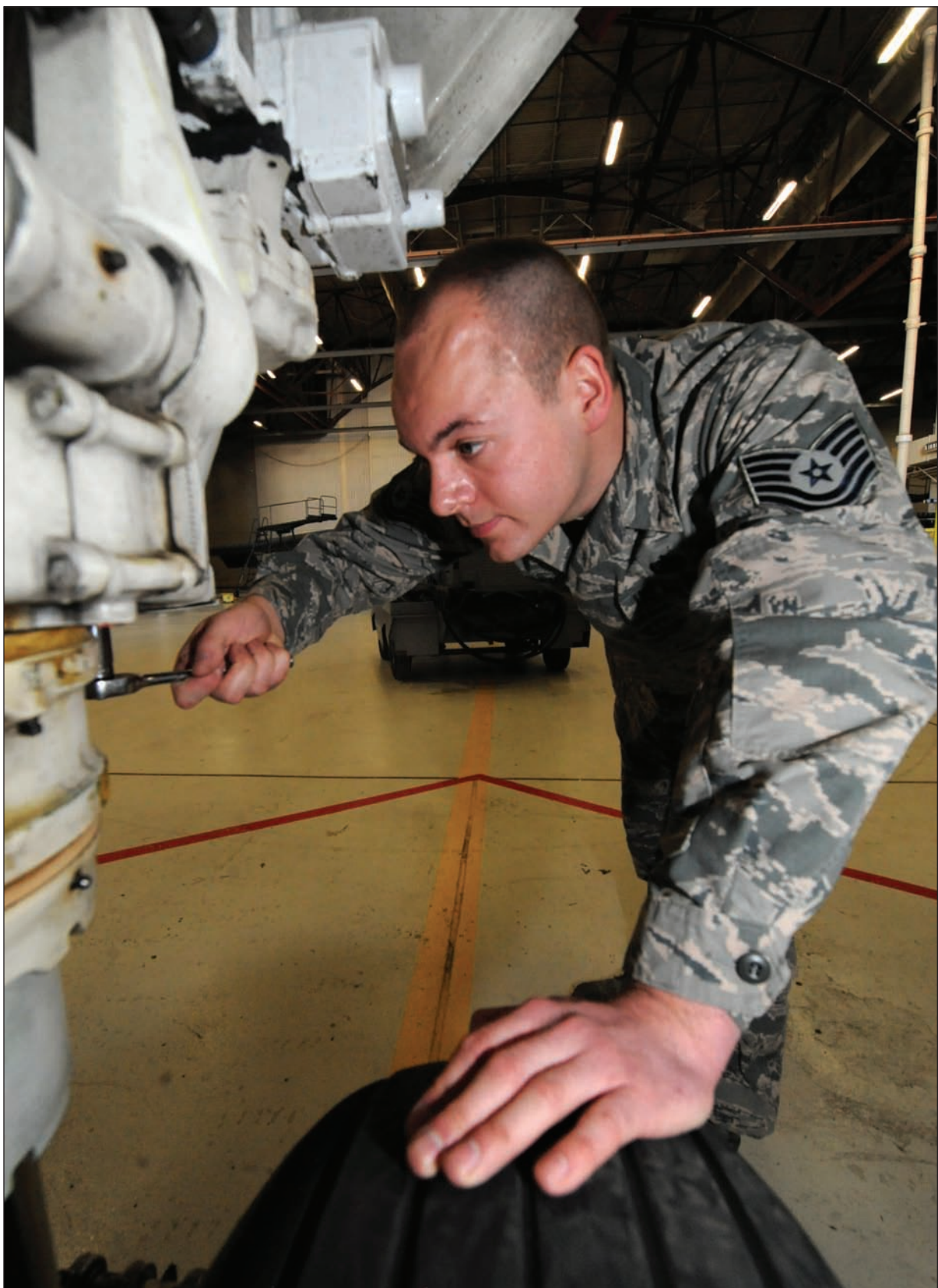
U.S. Air Force Tech Sgt. Aaron Bradley, a 393d Aircraft Maintenance Unit specialist section chief, uses a socket wrench to adjust the front landing gear of a B-2 Spirit at Whiteman Air Force Base, Mo., Feb. 18, 2016. When needed, Bradley wears a headset to communicate with a second member in the cockpit—who applies hydraulic pressure. This method allows the crew to adjust the steering of the front landing gear without actually turning the wheel, which prevents wear on the tires.
