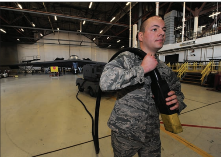
U.S. Air Force Tech Sgt. Aaron Bradley, a 393d Aircraft Maintenance Unit specialist section chief, prepares to supply power to a B-2 Spirit at Whiteman Air Force Base, Mo., Feb. 18, 2016. The power, provided by a generator, allows operation of the aircraft avionics system and is essential when working on the B-2's landing gear.
