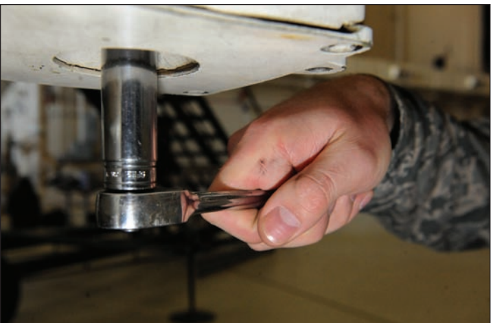
U.S. Air Force Tech. Sgt. Aaron Bradley, a 393d Aircraft Maintenance Unit specialist section chief, adjusts the front landing gear of a B-2 Spirit with a socket wrench at Whiteman Air Force Base, Mo., Feb. 18, 2016. A second member, located in the cockpit, communicates with Bradley through headsets, allowing the specialists to adjust the steering of the front landing gear without turning the wheel.
