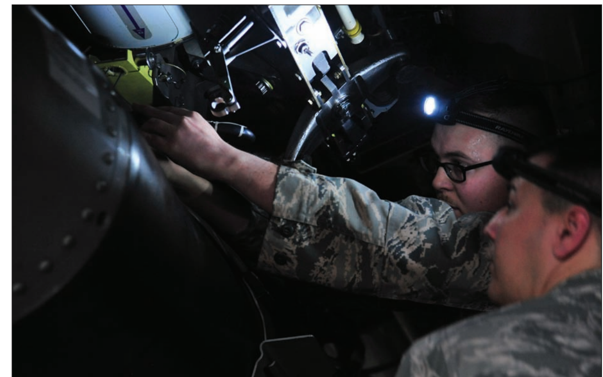
U.S. Air Force Tech. Sgt. Daniel Jensen, a load crew member assigned to the 131st Aircraft Maintenance Unit, secures the final trainer weapon for his team during the Annual Weapons Load Competition at Whiteman Air Force Base, Mo., Feb. 19, 2016. Each team must load two trainer weapons in addition to restocking all equipment before time is called.
