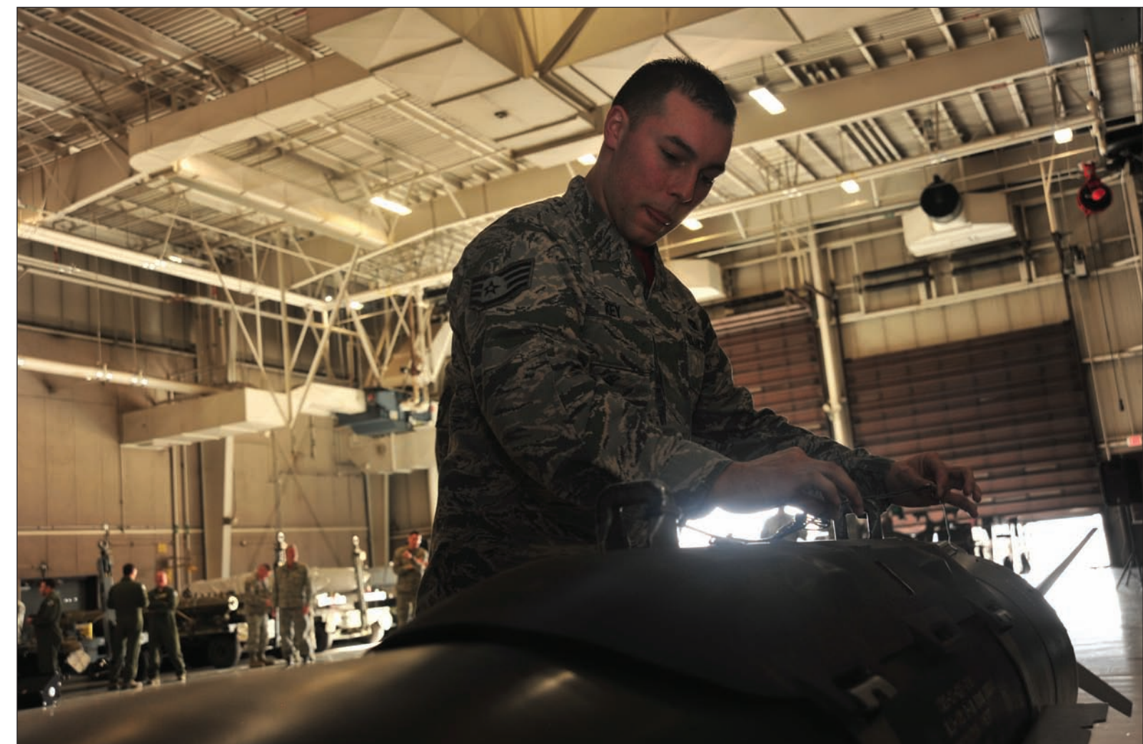
U.S. Air Force Staff Sgt. Jeremie Key, a load crew member assigned to the 131st Aircraft Maintenance Unit, surveys a trainer weapon during the Annual Weapons Load Competition at Whiteman Air Force Base, Mo., Feb. 19, 2016. Load crew members must check for damages on all munitions before they are loaded.
