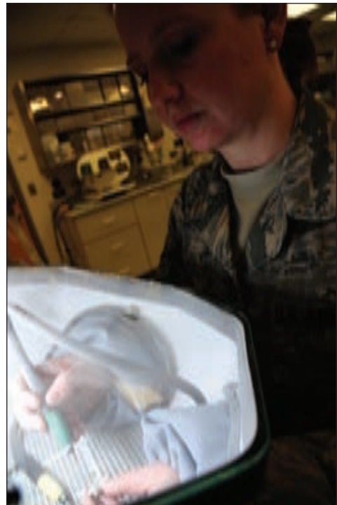
U.S. Air Force Staff Sgt. Melia Baxter, the 509th Medical Operations Squadron dental lab technician, prepares metal for a crown in the sand blast machine at Whiteman Air Force Base, Mo., Jan. 29, 2016. The sand blast machine cleans the metal for porcelain stacking, which is the process for making the crown resemble an actual tooth.
