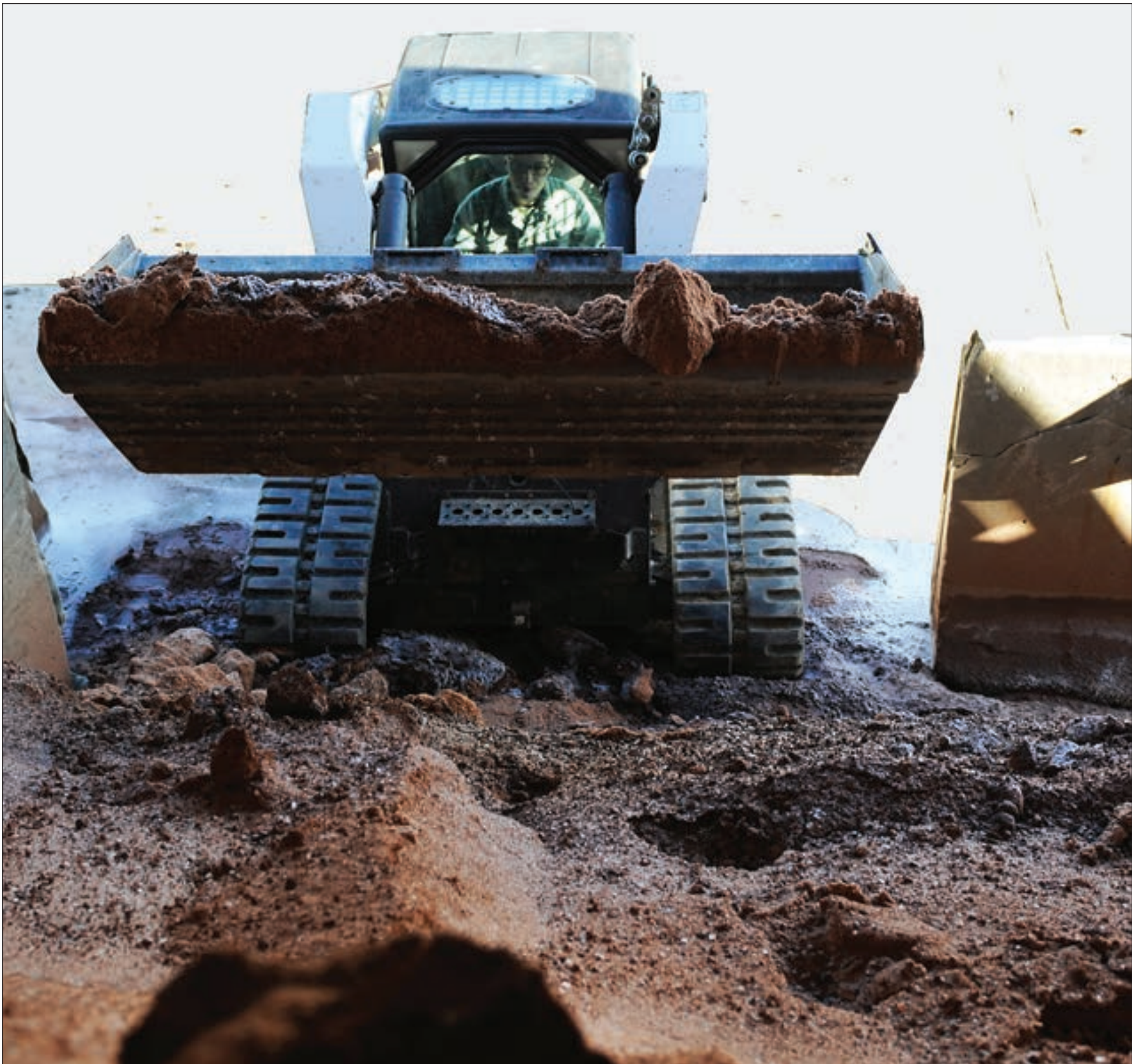
U.S. Air Force Senior Airman Glenn Cooley, a 509th Civil Engineer Squadron pavements and heavy equipment operator, uses a skid steer to transfer a deicing compound at Whiteman Air Force Base, Mo., Dec. 7, 2015. The mixture is used to melt ice on roads and parking lots.
