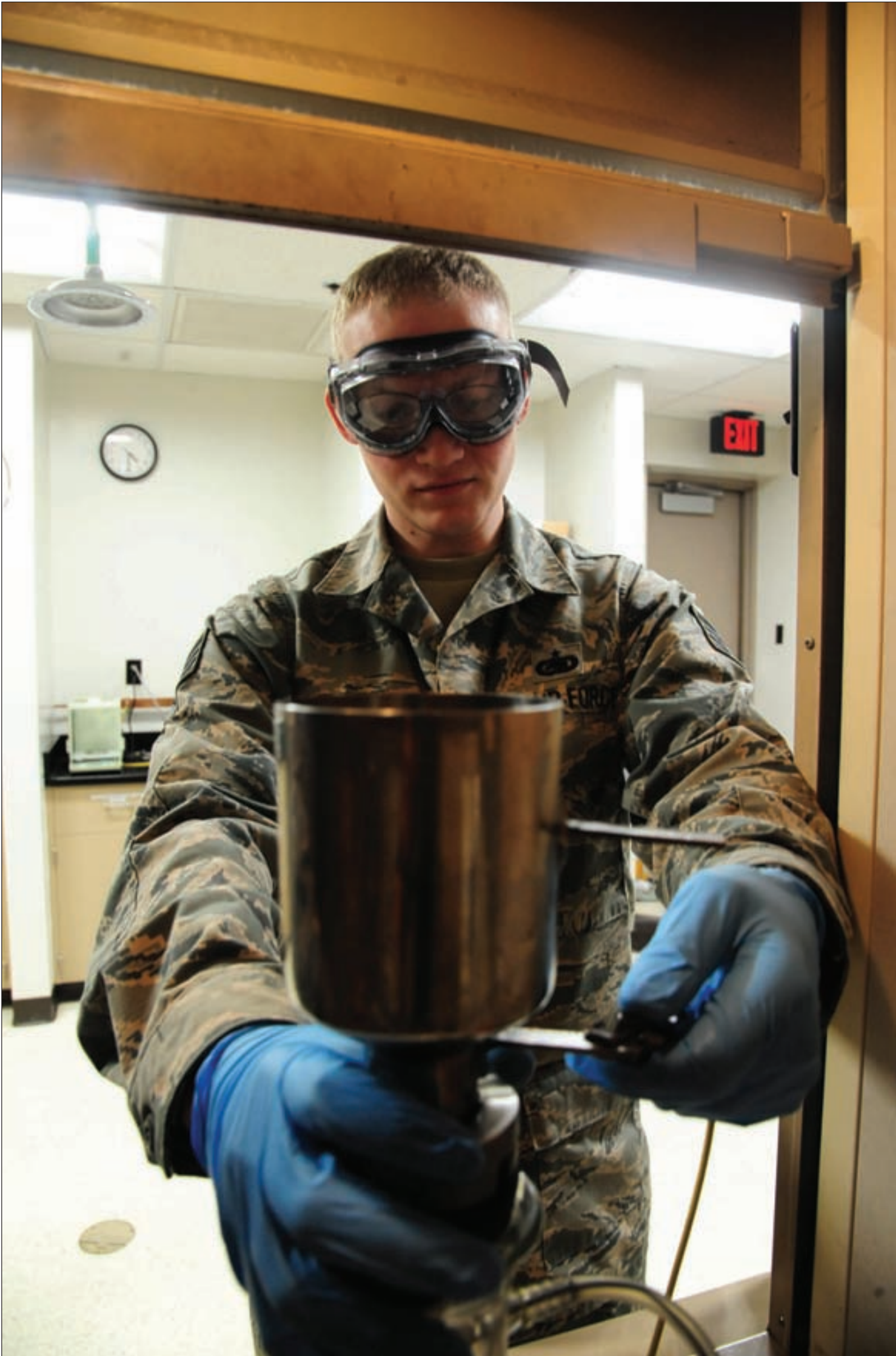
U.S. Air Force Staff Sgt. Nicholas Flamm, a 509th Logistics Readiness Squadron fuels service center operator, performs bottle method at Whiteman Air Force Base, Mo., Nov. 3, 2015. This process ensures all potential contaminants of the fuel are processed through the filter and do not settle to the bottom of the sample container.
