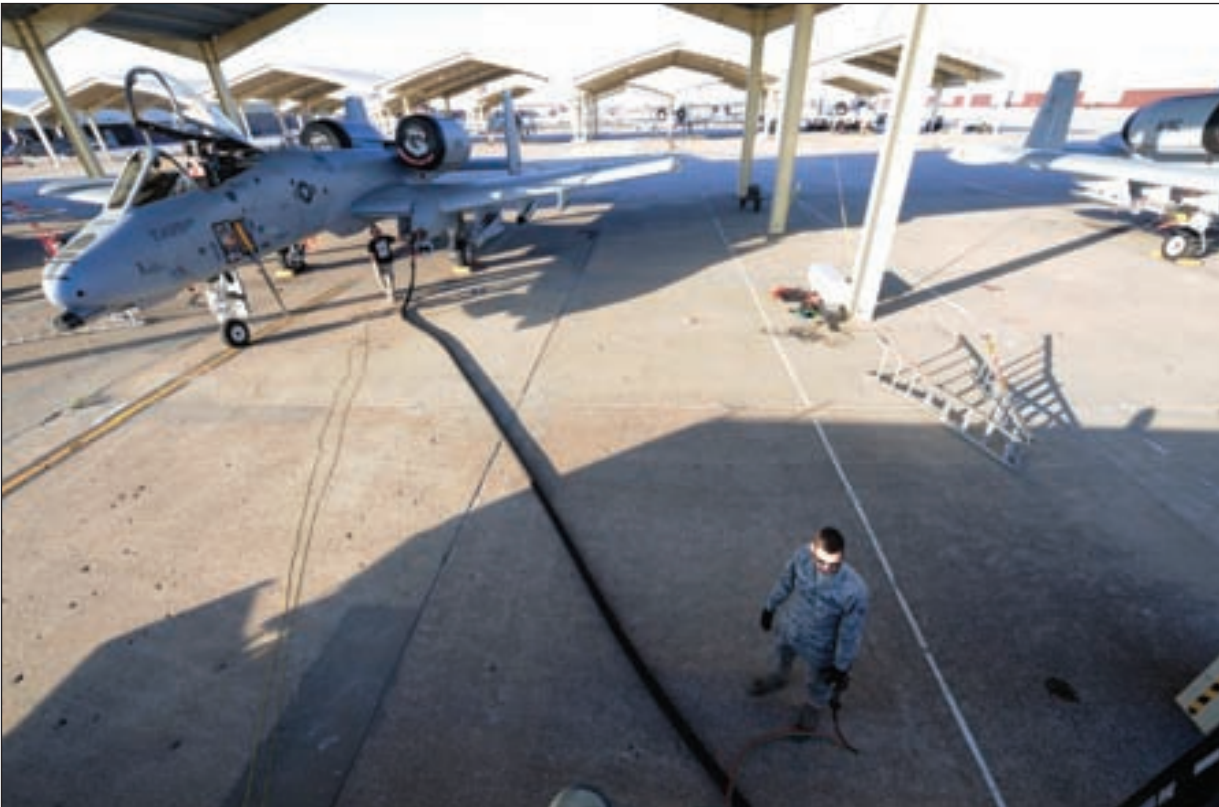
U.S. Air Force Airman 1st Class Jacob McSheffrey, a 509th Logistics Readiness Squadron fuels distribution operator, fuels an A-10 Thunderbolt II at Whiteman Air Force Base, Mo., Nov. 3, 2015. The fuels shop mission is to ensure aircraft, vehicles and equipment receive clean, dry fuel with no contaminants to assist members in accomplishing tasks. (U.S. Air Force photo by Senior Airman Keenan Berry)
