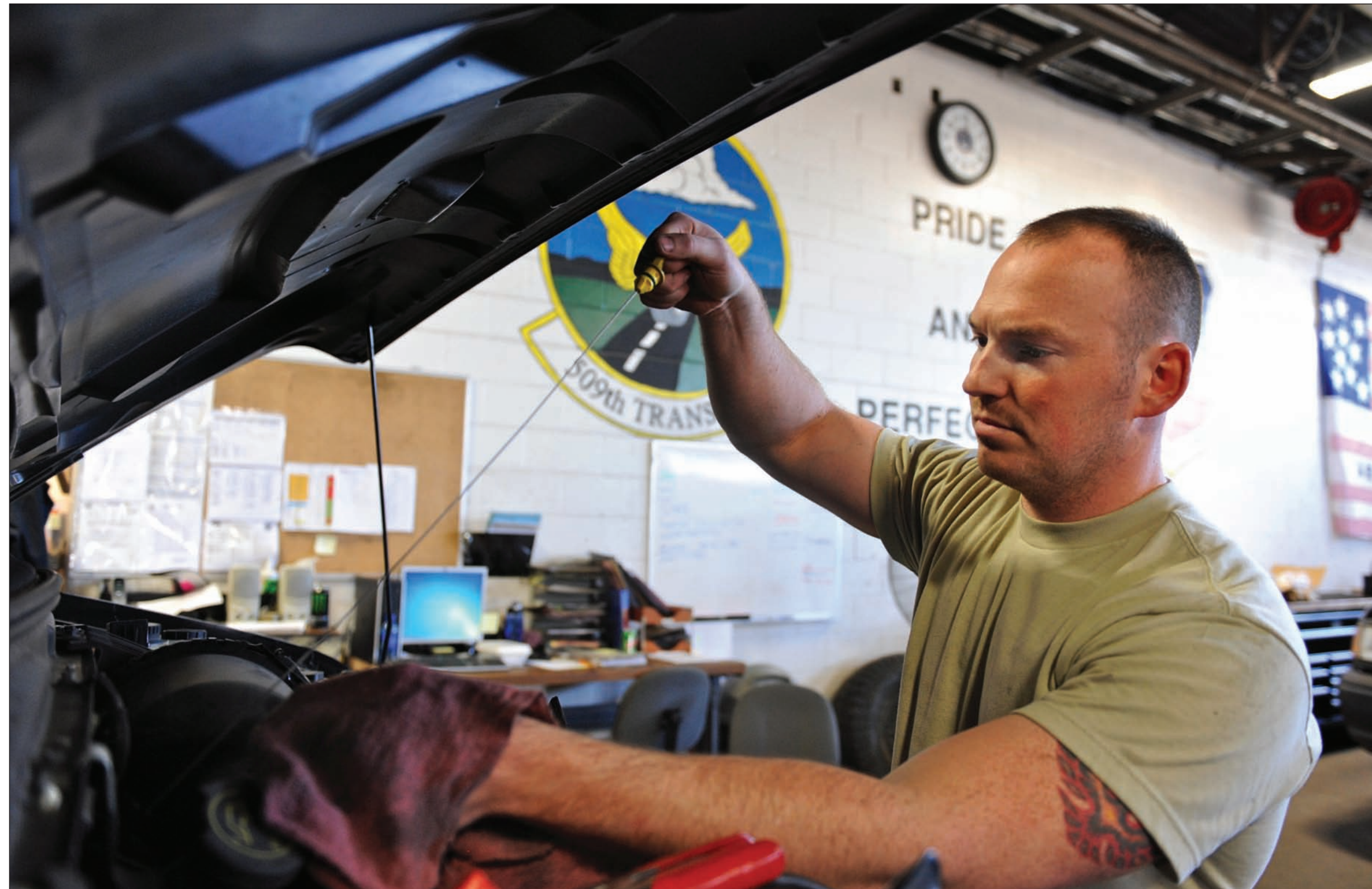
U.S. Air Force photo/Airman 1st Class Michaela R. Slanchik Senior Airman Jeremy Lee, 509th Logistics Readiness Squadron general purpose mechanic, checks the transmission fluid levels in a government vehicle at Whiteman Air Force Base, Mo., Oct. 26, 2015. Preventative maintenance such as checking fluid levels, tire pressure and tread are some of many duties vehicle maintainers perform to ensure the base's fleet of vehicles is fully operational.
